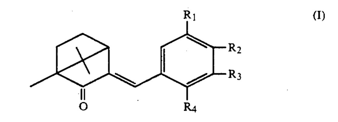
where R<sub>1</sub> denotes H, OH, C<sub>1</sub>-C<sub>3</sub> alkyl or C<sub>1</sub>-C<sub>8</sub> alkoxy, R<sub>3</sub> denotes OH, C<sub>1</sub>-C<sub>3</sub> alkyl or C<sub>1</sub>-C<sub>8</sub> alkoxy, or else when R<sub>1</sub> denotes H or OH, R<sub>3</sub> can represent C<sub>1</sub>-C<sub>8</sub> alkyl, R<sub>2</sub> and R<sub>4</sub> denote H or OH, at least one of the radicals R<sub>2</sub> and R<sub>4</sub> representing OH.
