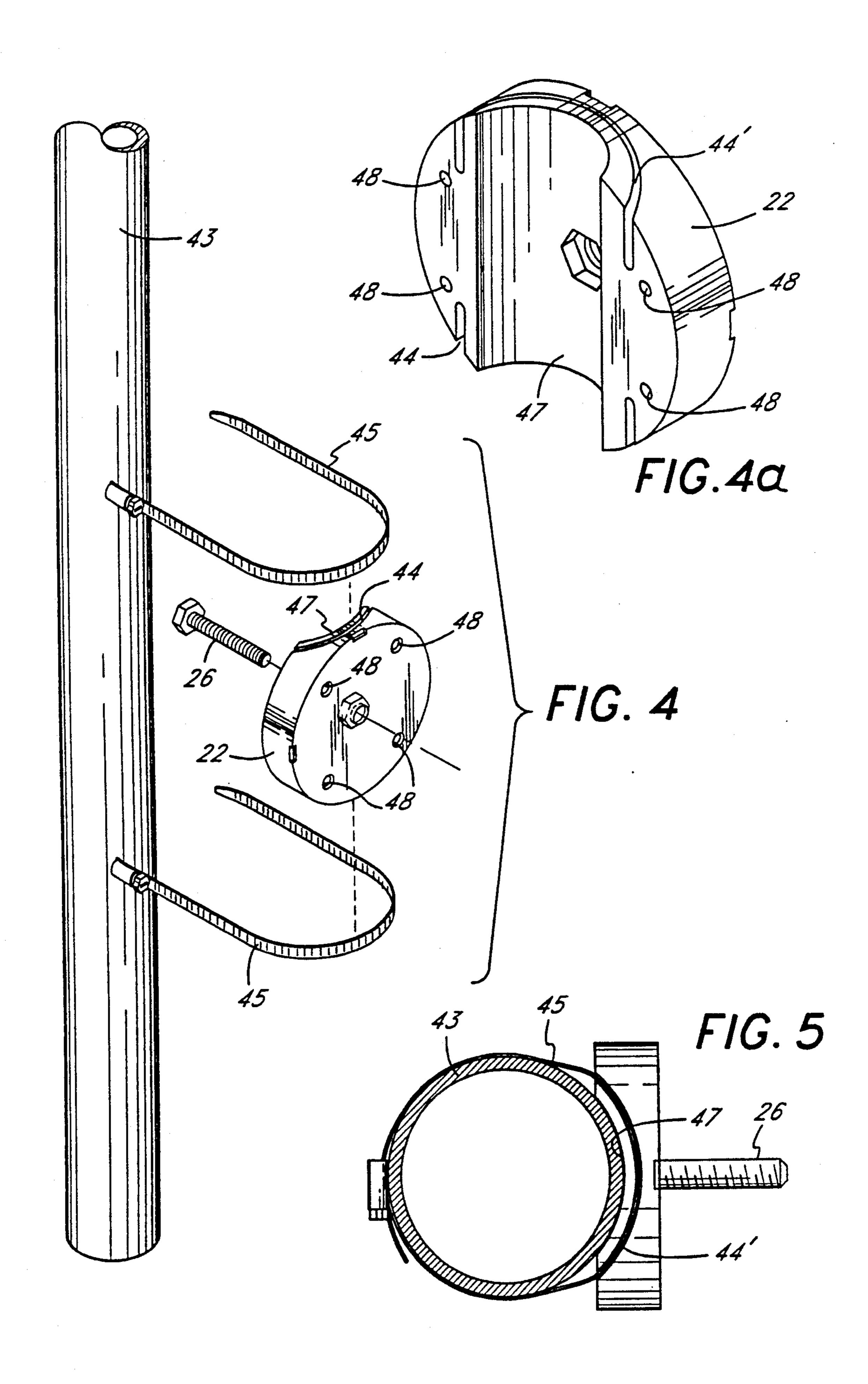
FIG. 5 is a cross-sectional top view of the base and clamp assembly of FIG. 4.
