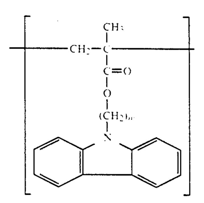
where m is an integer of from 3 to 11. The novel methacrylate (co)polymers containing carbazolyl side groups can advantageously be used as photoconductors in photoconductive layers, in particular of electrophotographic recording elements.
