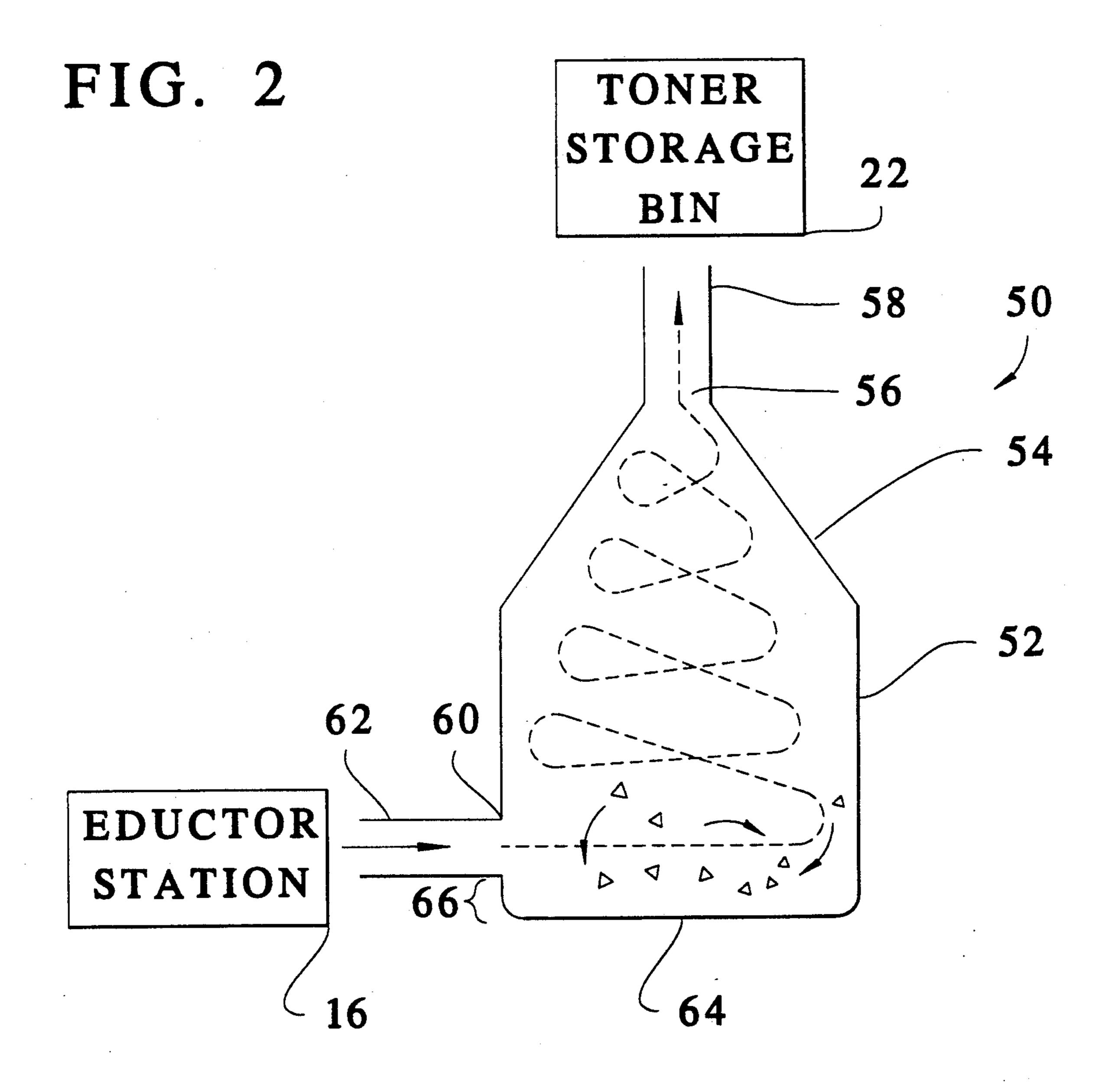
a flow adjusting air current layer interposed between walls defining the main and subsidiary passages and the particular material conveyed by the air currents.
