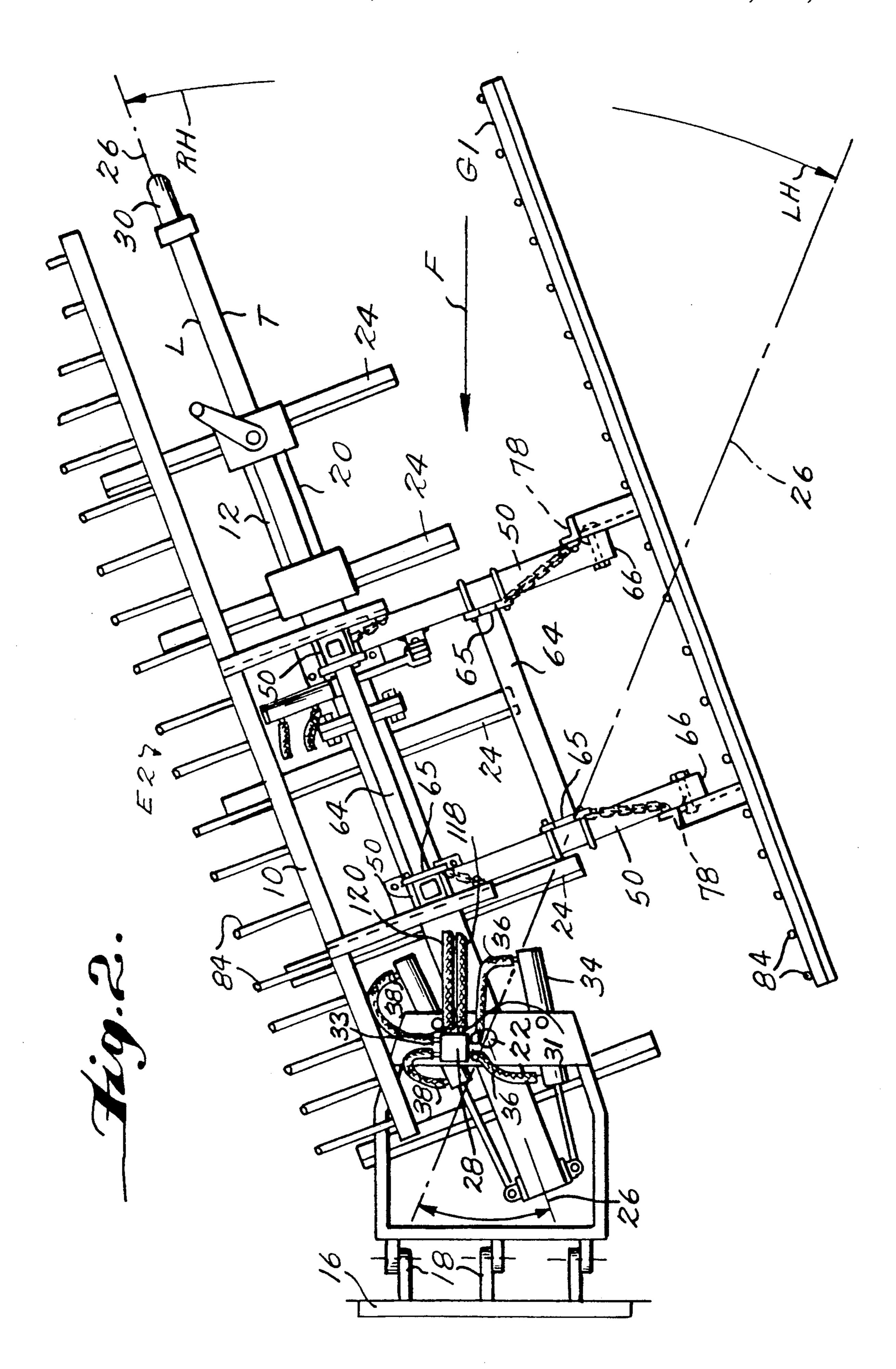
tine bar allows the tine bar to swing out of the way of hard debris.
