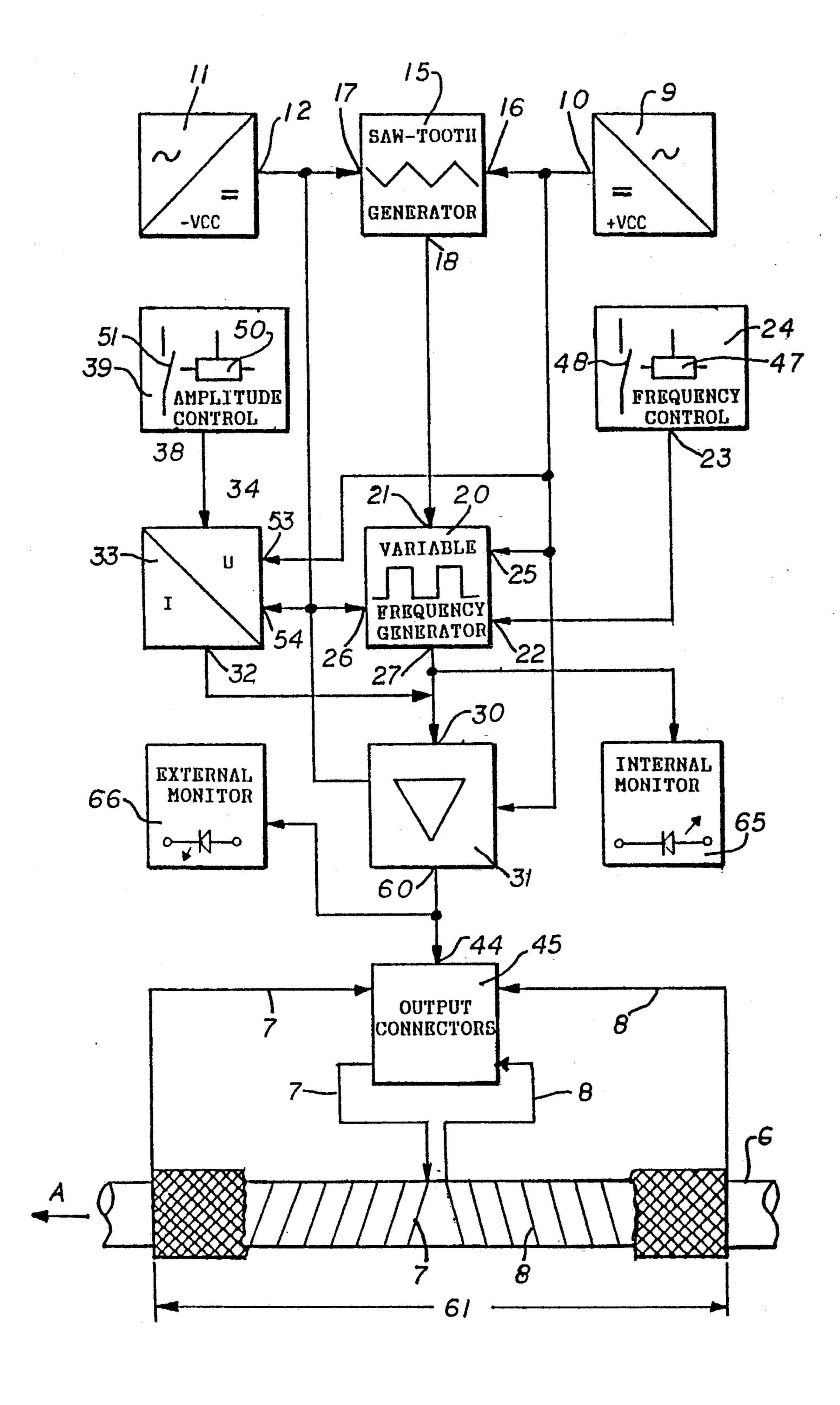
ELECTRONIC LIME CONTROLLER WITH CONTROLS RESPONSIVE TO FLOW RATES AND WATER HARDNESS
