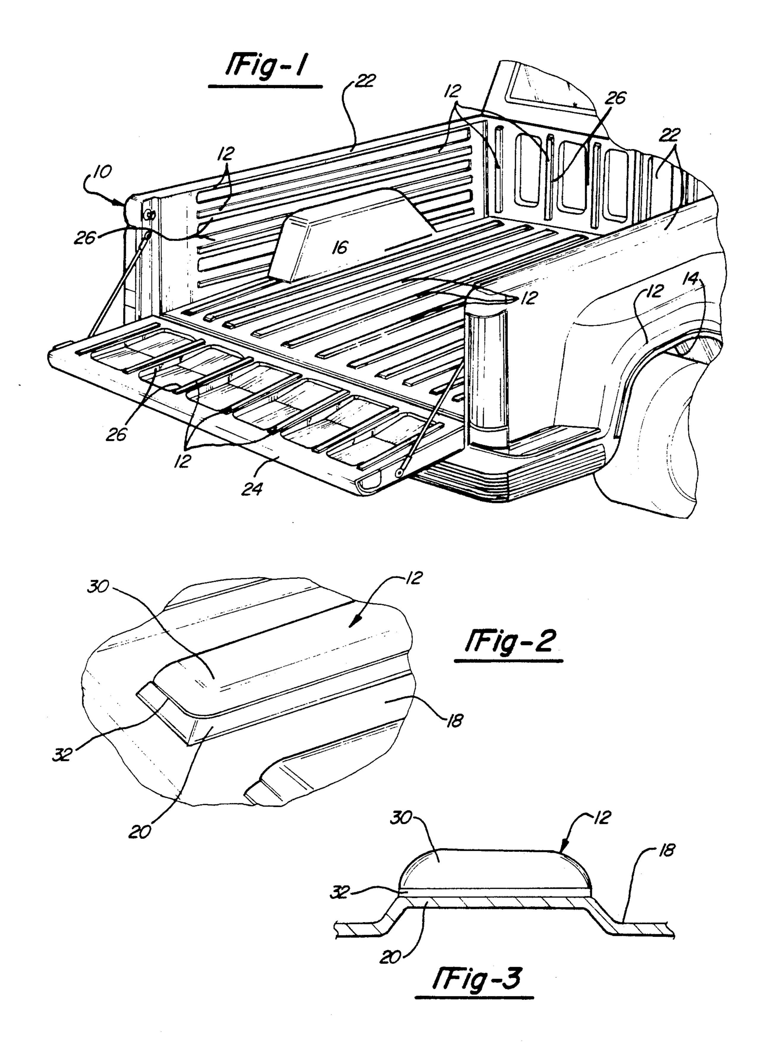
backing adhesive maintains the position of the molding while its elastomeric properties absorb any impacts returning to its original configuration.
