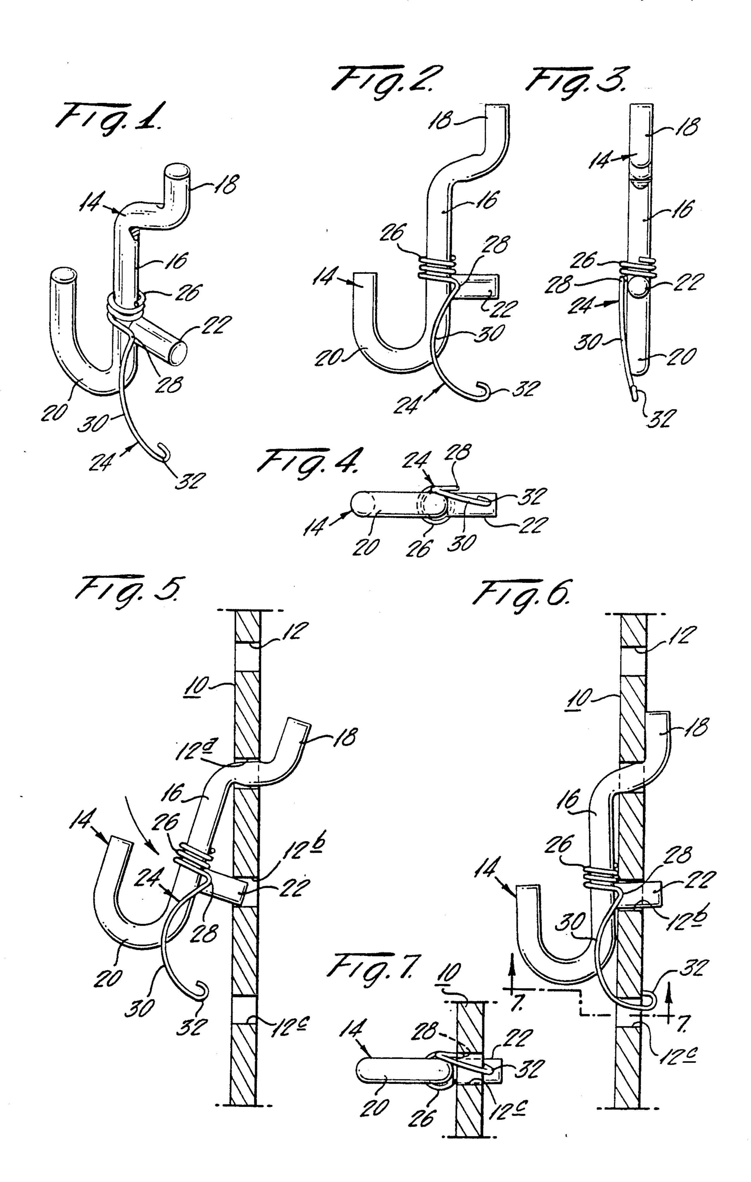
It is accordingly a first object of the invention to provide a clip for securing a toolholder in position on a pegboard and particularly for preventing dislodgment
