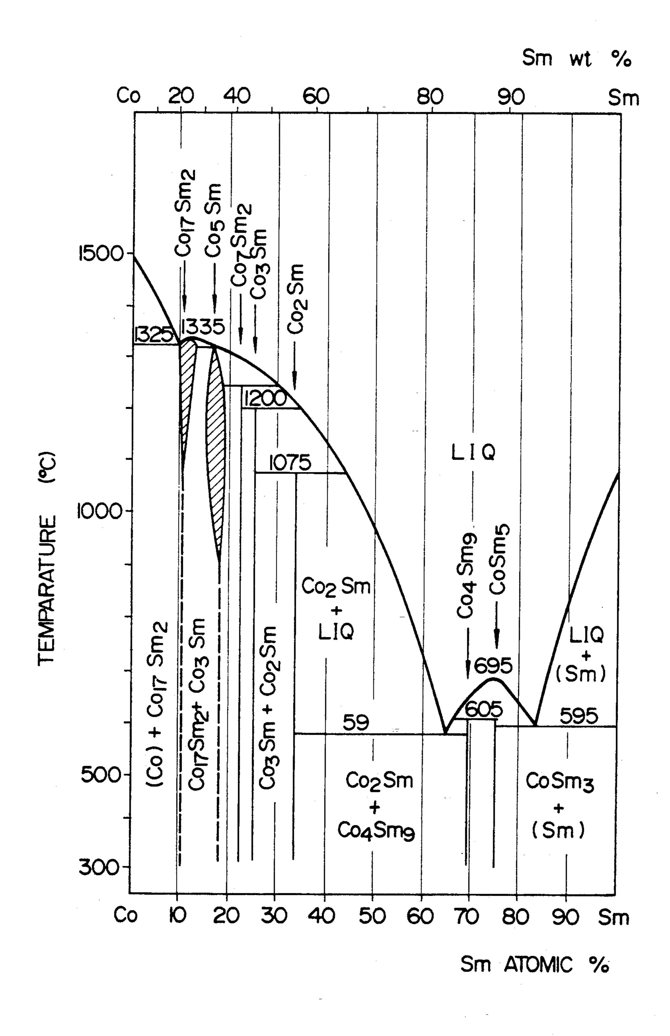
RARE EARTH PERMANENT MAGNET, METHOD OF HEAT TREATMENT OF SAME, AND MAGNET BODY
