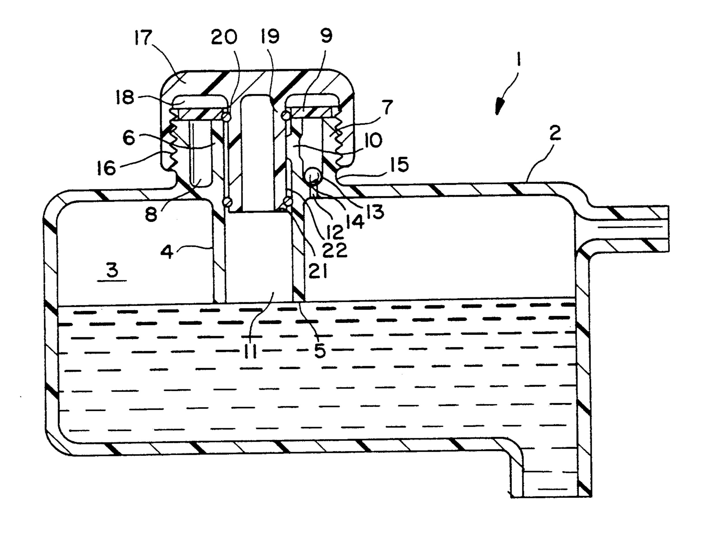
the second sealed boundary is closed when the cap is only partially opened.
