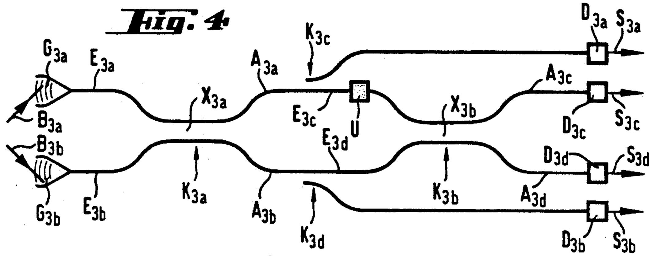
APPARATUS AND METHOD HAVING AT LEAST ONE WAVEGUIDE COUPLER TO CREATE AT LEAST TWO SIGNALS HAVING A MUTUAL PHASE SHIFT NOT EQUAL TO 180 DEGREES
