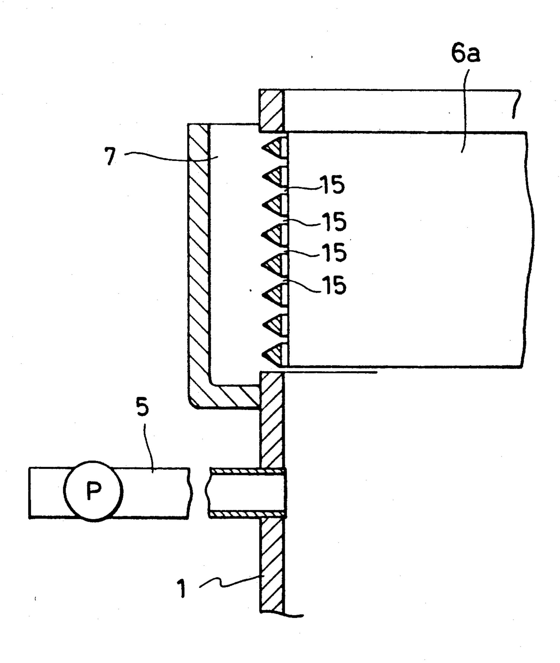
adapted to rub the inner surface of aforementioned outer peripheral wall and prevent the slits from the clogging. The brushes, however, fail to manifest fully
