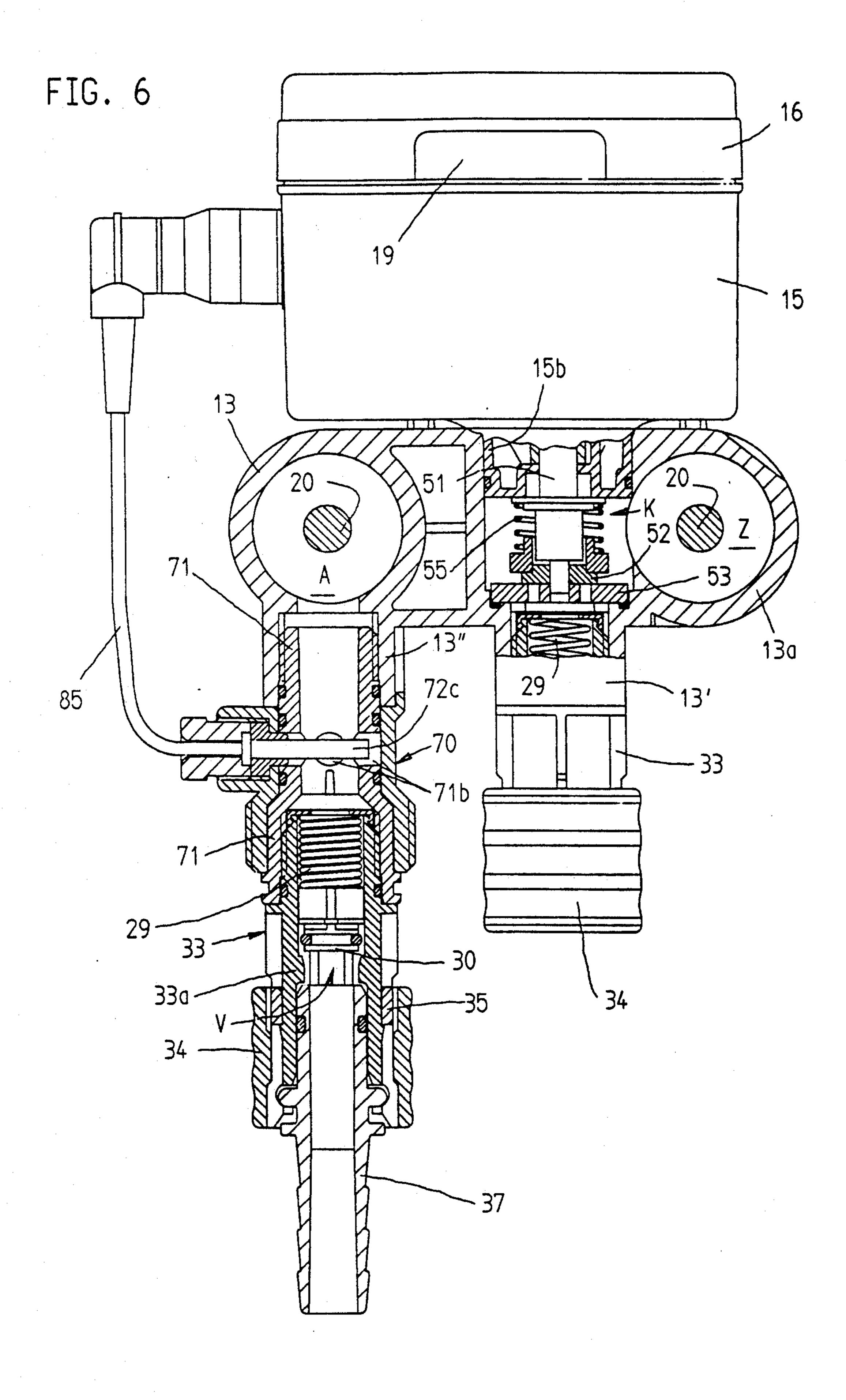
mounted on each of said fittings, and at least one of said fittings is adapted to be provided with monitoring means, which are connected between the tubular port which communicates with the return passage section of said one fitting and the associated hose coupling.
