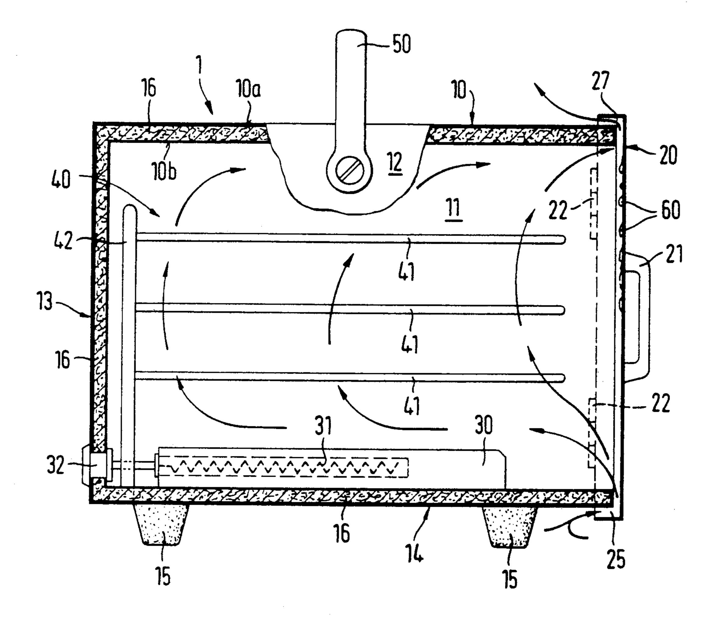
substantially at ambient temperature so that it acts as a condensate trap for the moisture-saturated air which flows therepast, at least a substantial part of the moisture entrained in the air being deposited as condensate on that part of the side wall of the container. When there is a sufficient amount of condensate, it can be
