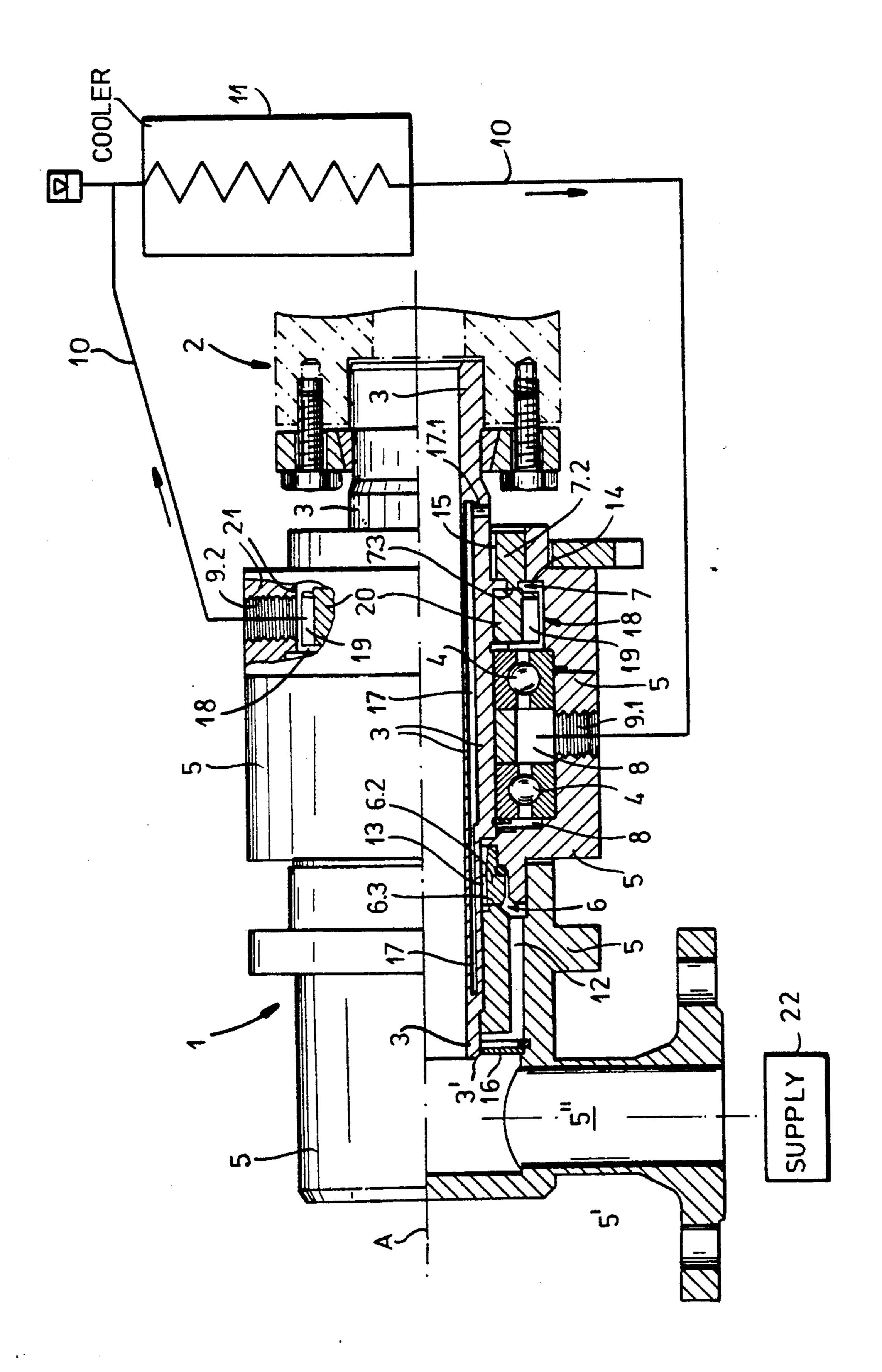
COUPLING FOR FEEDING A HEAT-EXCHANGE MEDIUM TO A ROTATING BODY
