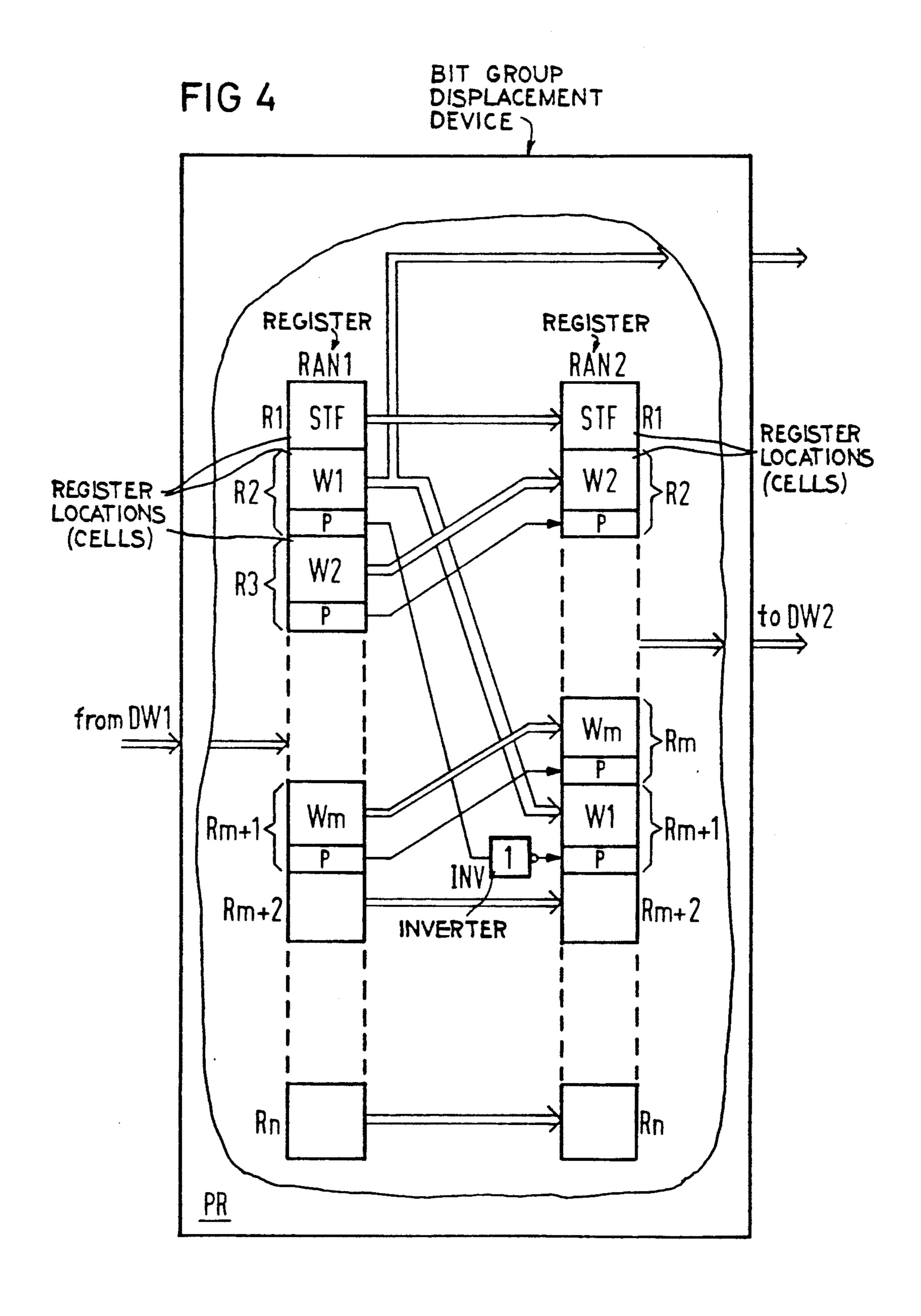
METHOD AND CIRCUIT ARRANGEMENT FOR THE ACCEPTANCE AND FORWARDING OF MESSAGE CELLS TRANSMITTED ACCORDING TO AN ASYNCHRONOUS TRANSFER MODE BY AN ASYNCHRONOUS TRANSFER MODE SWITCHING EQUIPMENT
