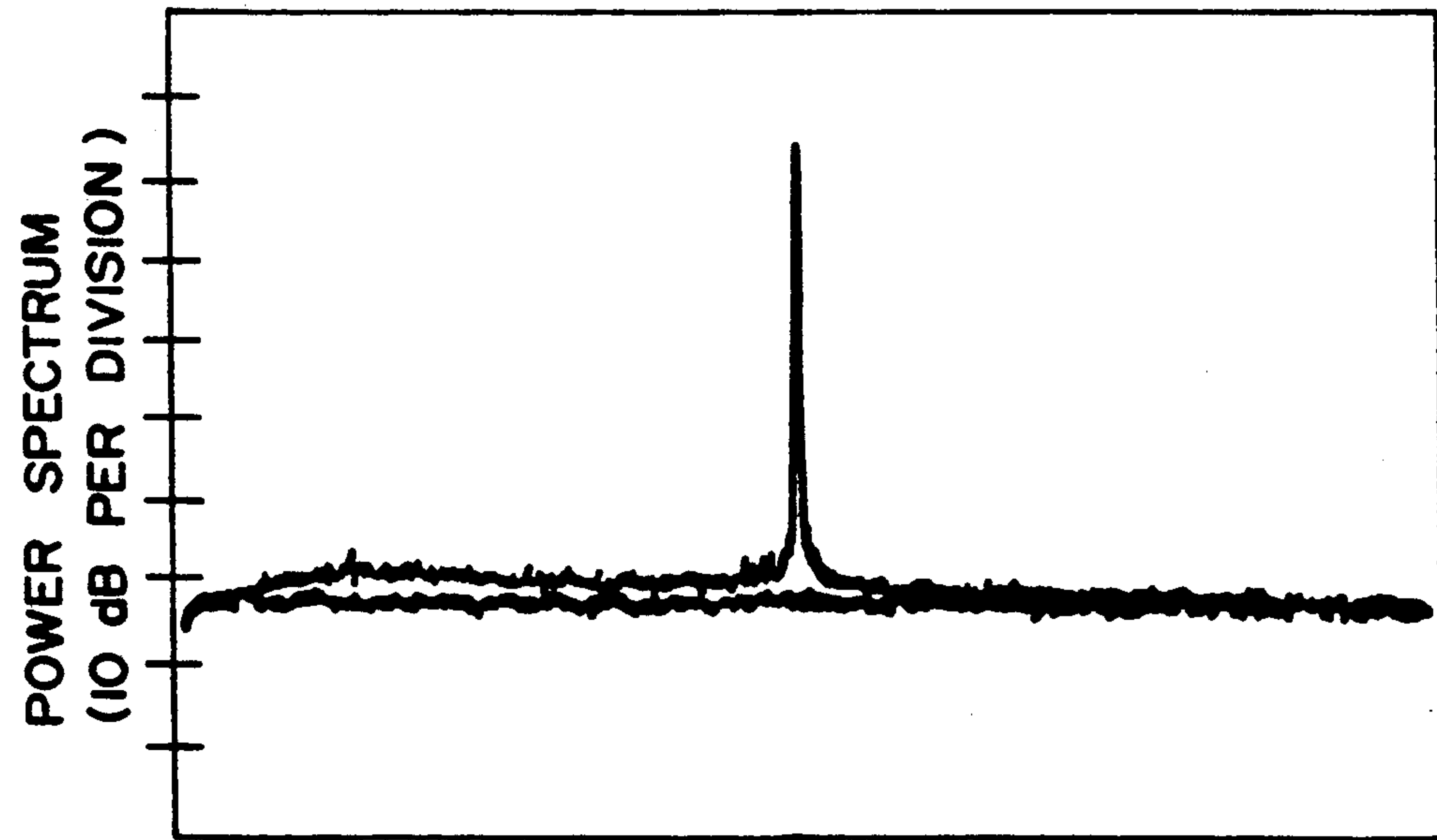
FREQUENCY CoNiPt SPUTTERED ON SPUTTERED Ni 2 P LAYER 500 Å IN THICKNESS
