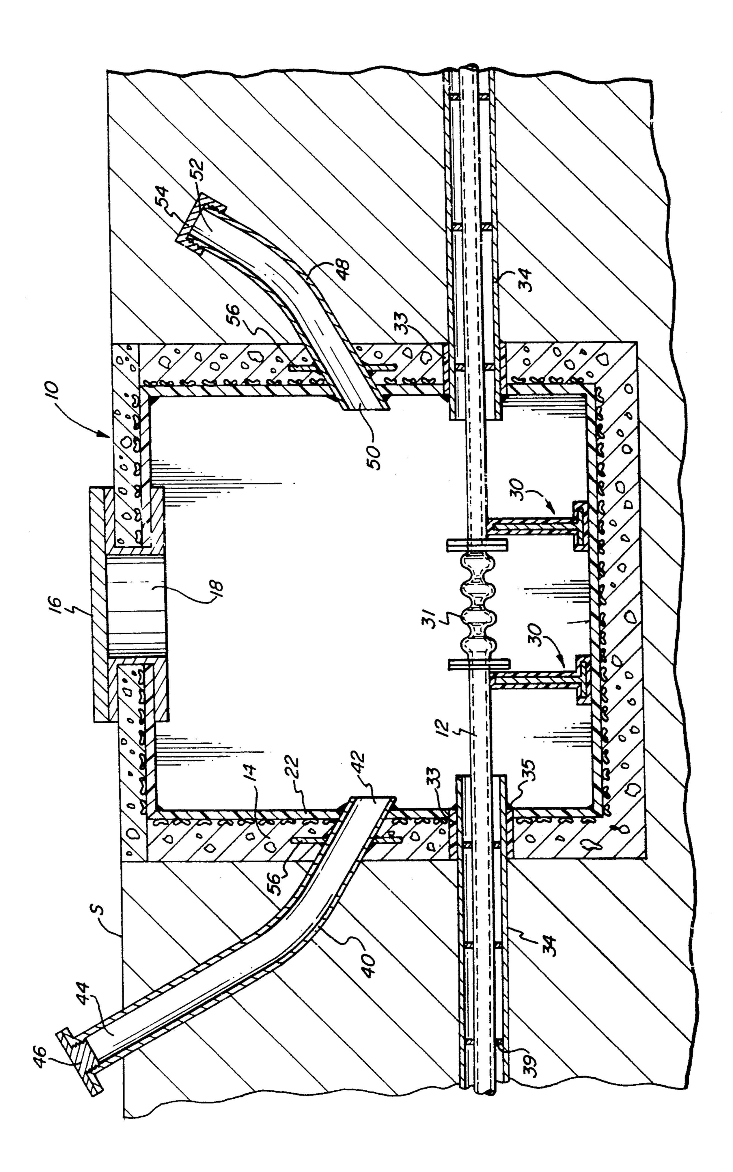
terminated inside of the lined-concrete tanks or housings. The tanks are designed to allow straight lengths of primary piping between consecutive tank locations.
