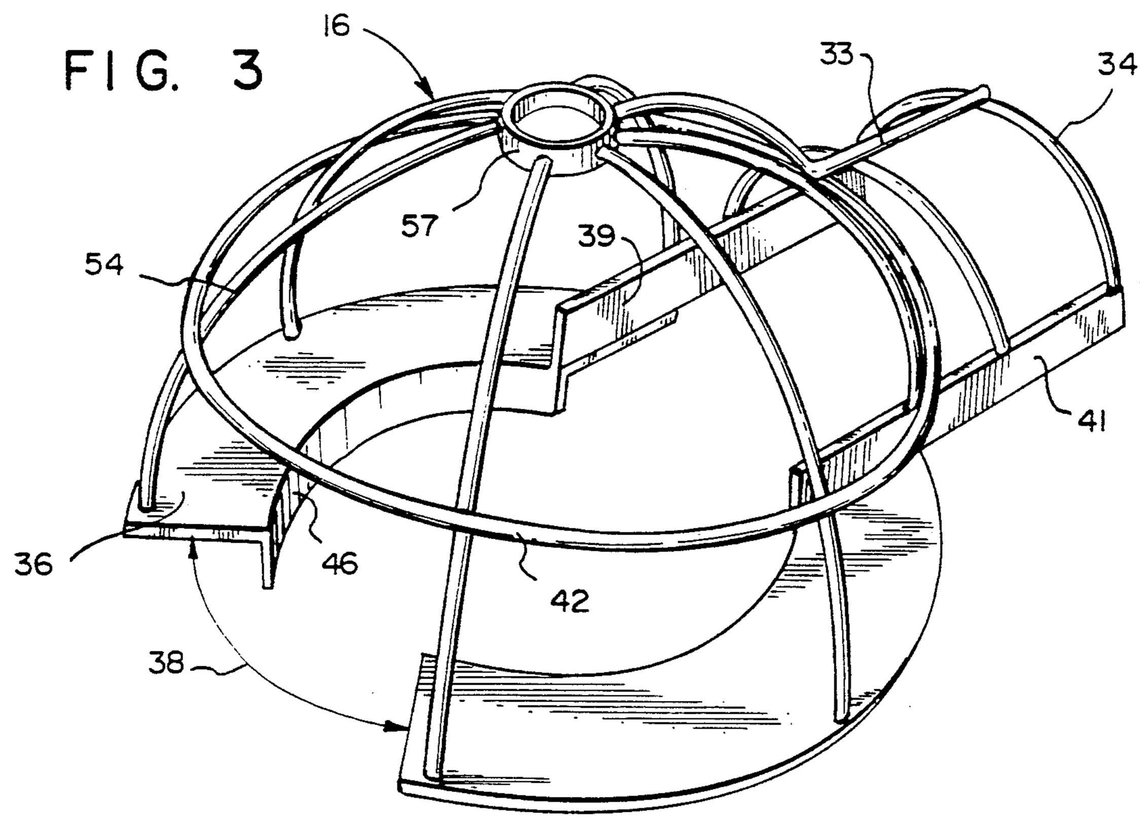
PROVISIONAL PROTECTIVE MEANS FOR PIT VALVE CASING
