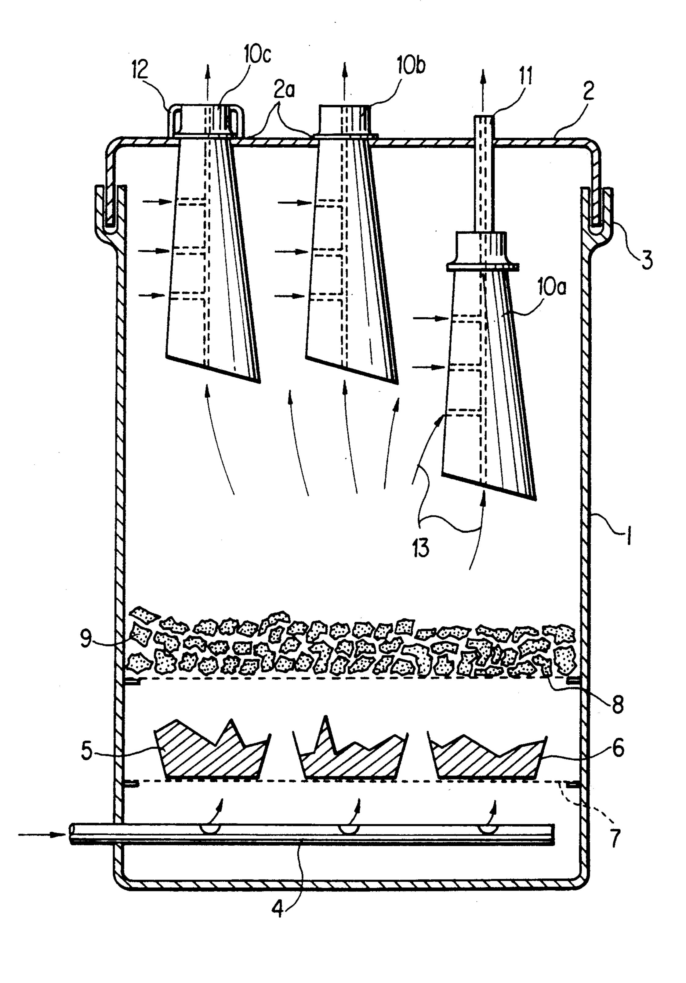
PROCESS AND APPARATUS FOR THE SIMULTANEOUS DEPOSITION OF A PROTECTIVE COATING ON INTERNAL AND EXTERNAL SURFACES OF HEAT-RESISTANT ALLOY PARTS
