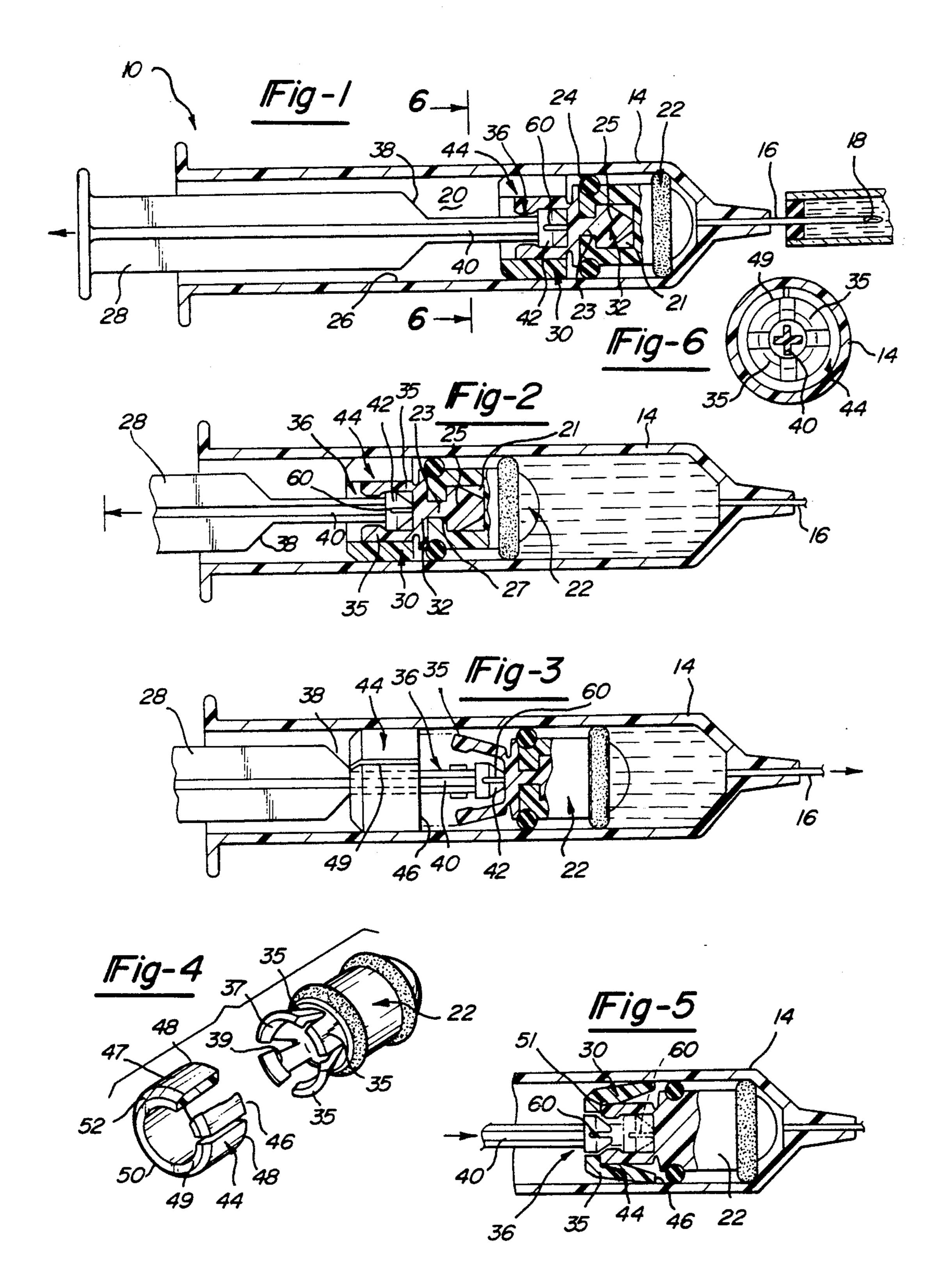
forward so that the plunger can only be pushed forward toward the needle and cannot thereafter be drawn away from the needle a second time. If the plunger rod is pulled a second time, it is disconnected from the
