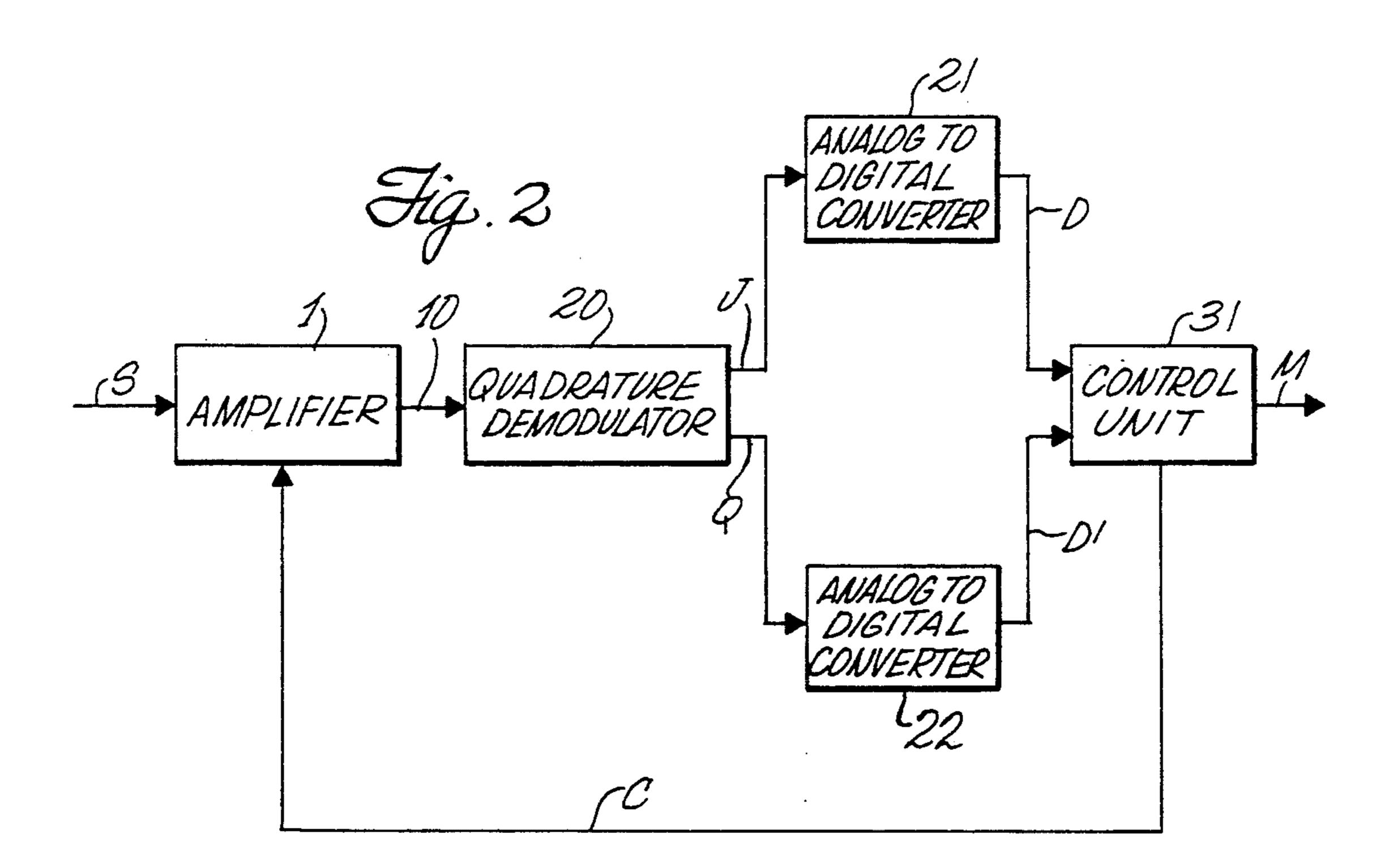
DIGITAL MEASURING CIRCUIT FOR MEASURING AN ELECTRICAL SIGNAL
