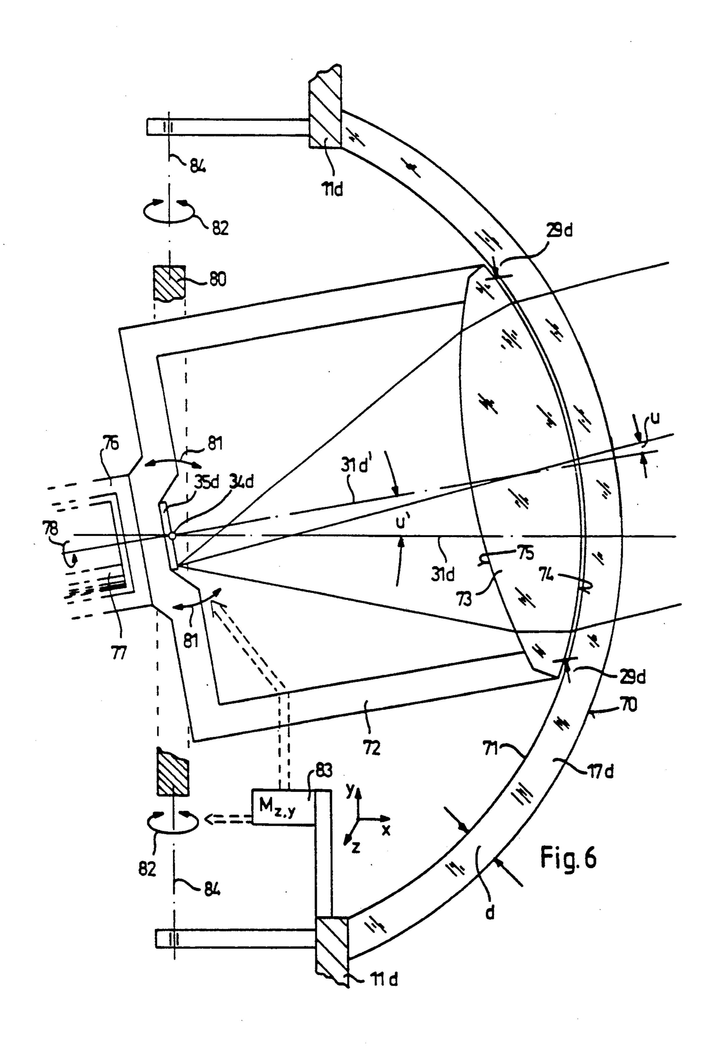
The invention concerns an underwater vehicle with a 5 passive optical observation system, equipped with an observation window which has a diameter ranging from
