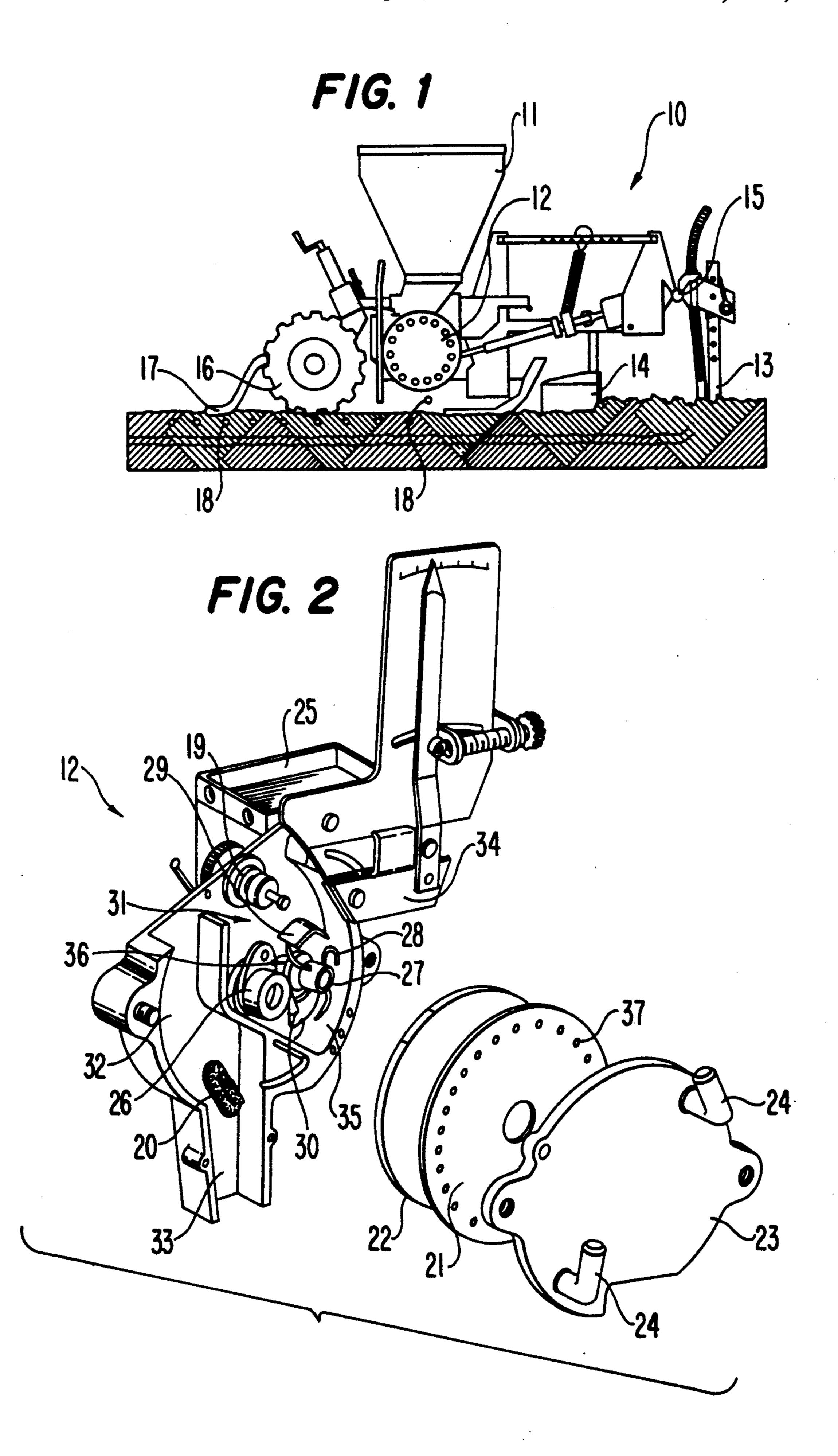
DEVICE TO STIR AND FEED SEEDS FOR PNEUMATIC DISTRIBUTORS OR SOWING **MACHINES**
