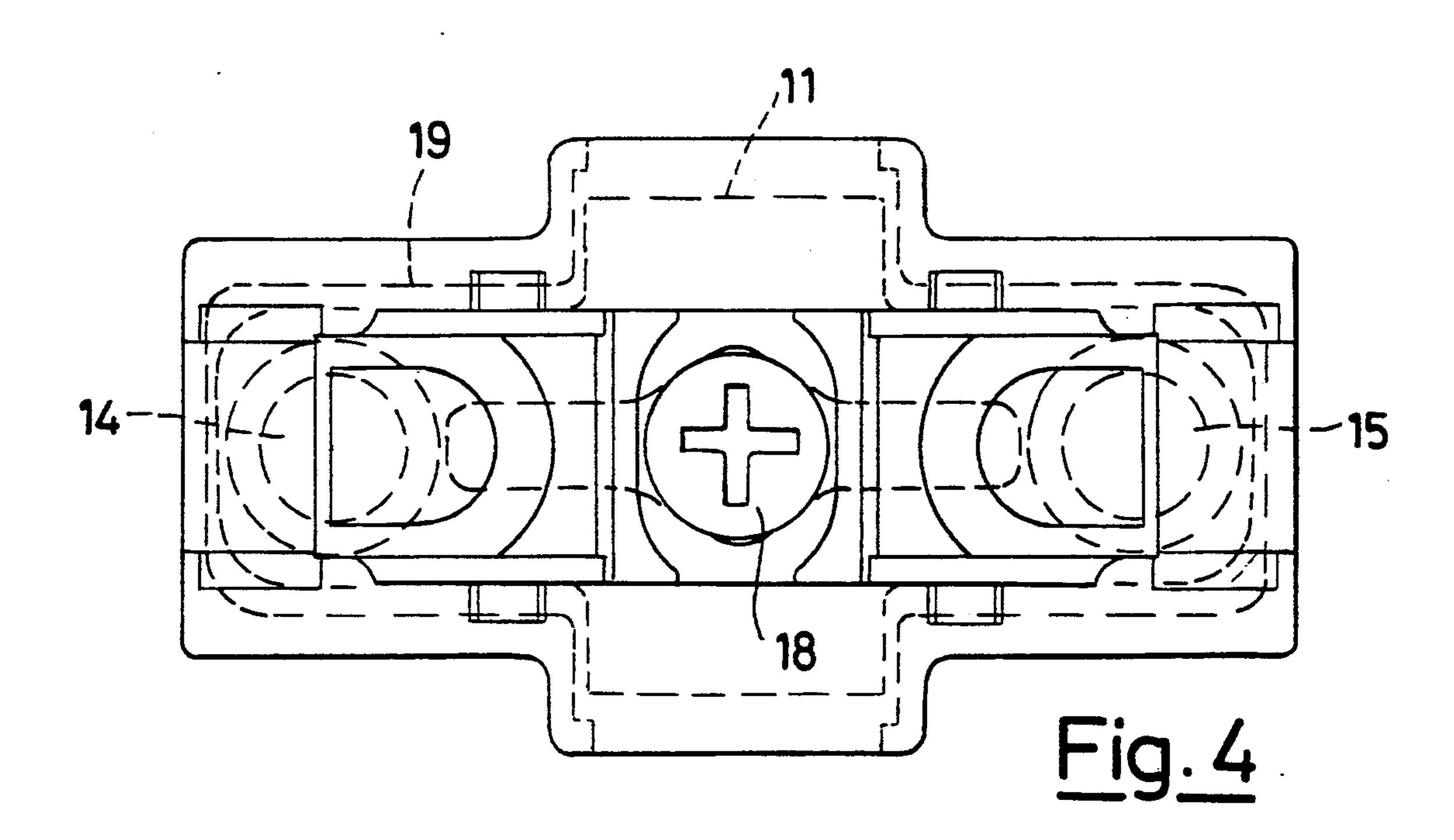
BASE WITH ADJUSTABLE ELEMENTS FOR A HINGE WING
