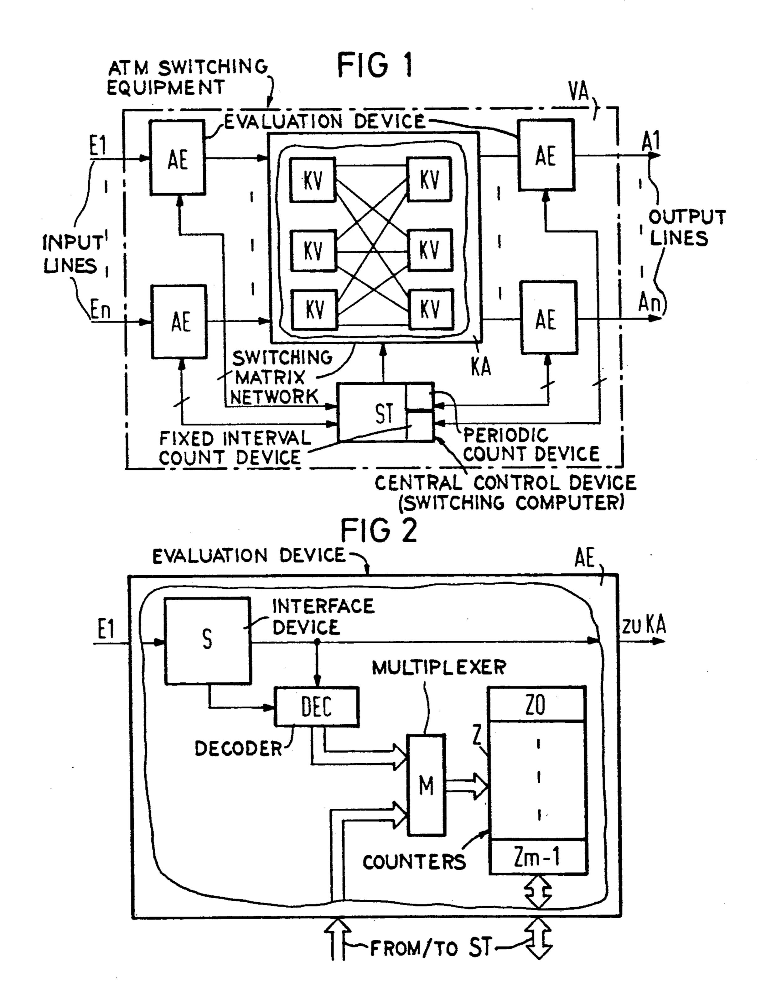
METHOD AND CIRCUIT ARRANGEMENT FOR DETERMINING THE QUALITY OF VIRTUAL CONNECTIONS THROUGH AN ASYNCHRONOUS TRANSFER MODE SWITCHING EQUIPMENT
