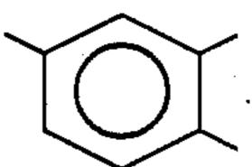
The A<sup>2</sup> radicals may be aromatic hydrocarbon or substituted aromatic hydrocarbon radicals, with illustrative substituents being alkyl, cycloalkyl, alkenyl (e.g., crosslinkable-graftable moieties such as allyl), halo (especially fluoro, chloro and/or bromo), nitro and alkoxy.
