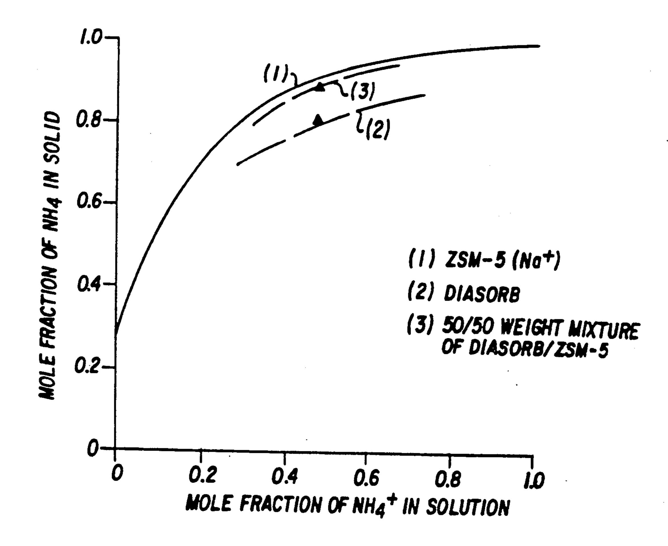
FIG. 2 NH4+-NO+ EXCHANGE ISOTHERMS AT 25°C
