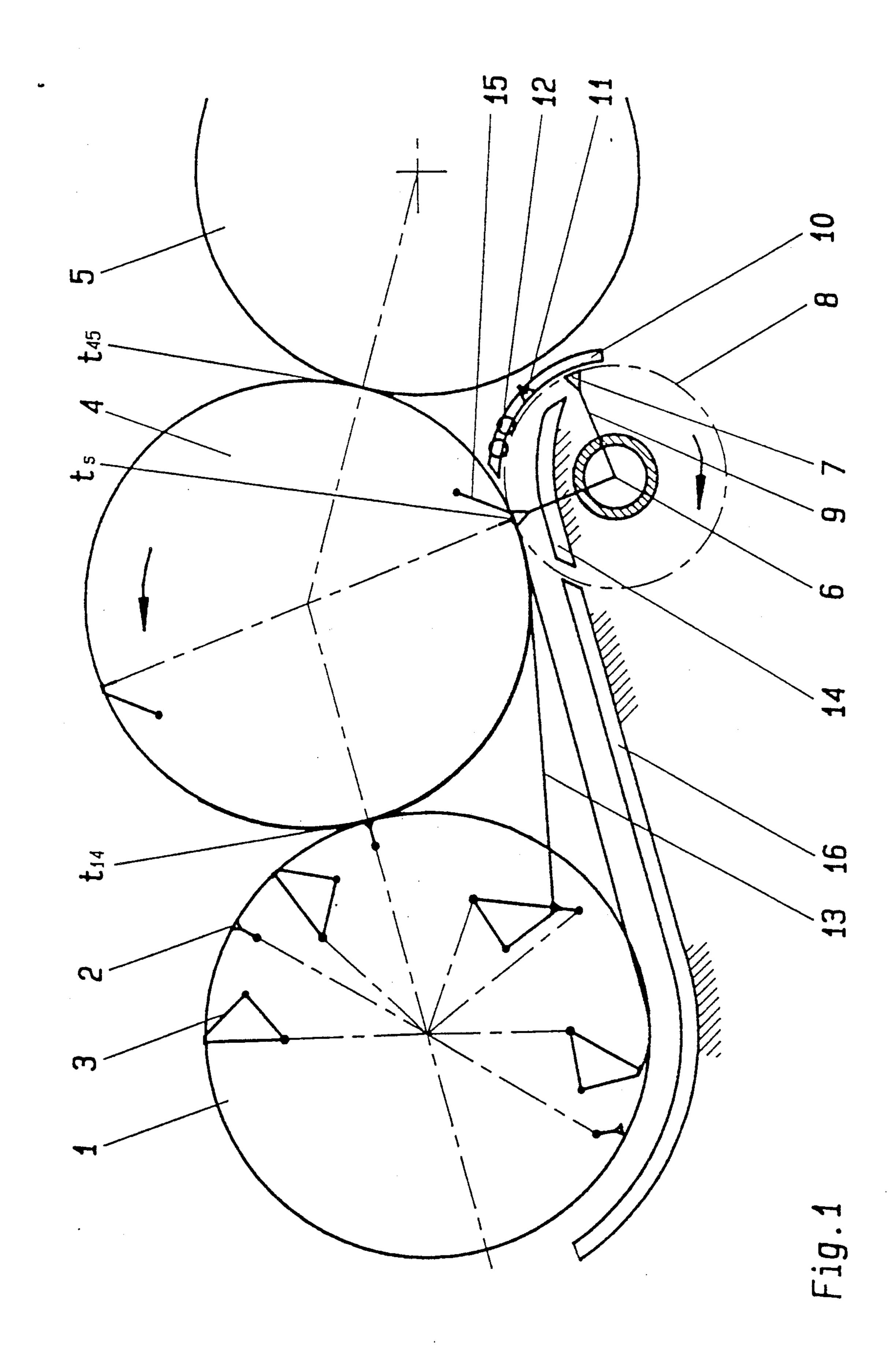
SHEET FEEDING UNIT FOR ROTARY PRINTING MACHINE
