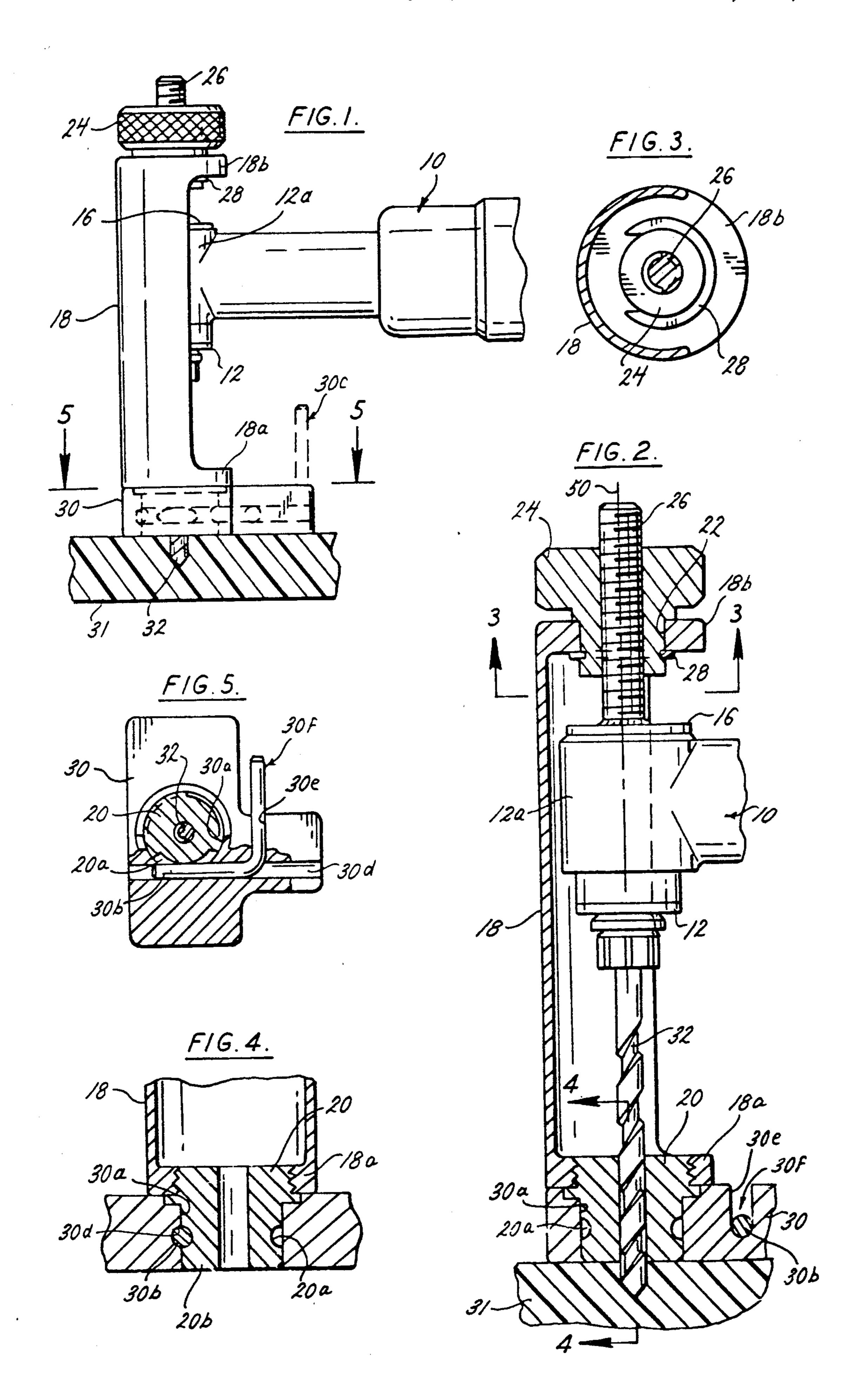
low torque on the knurled screw support to be converted to high axial thrust on the drill assembly.
