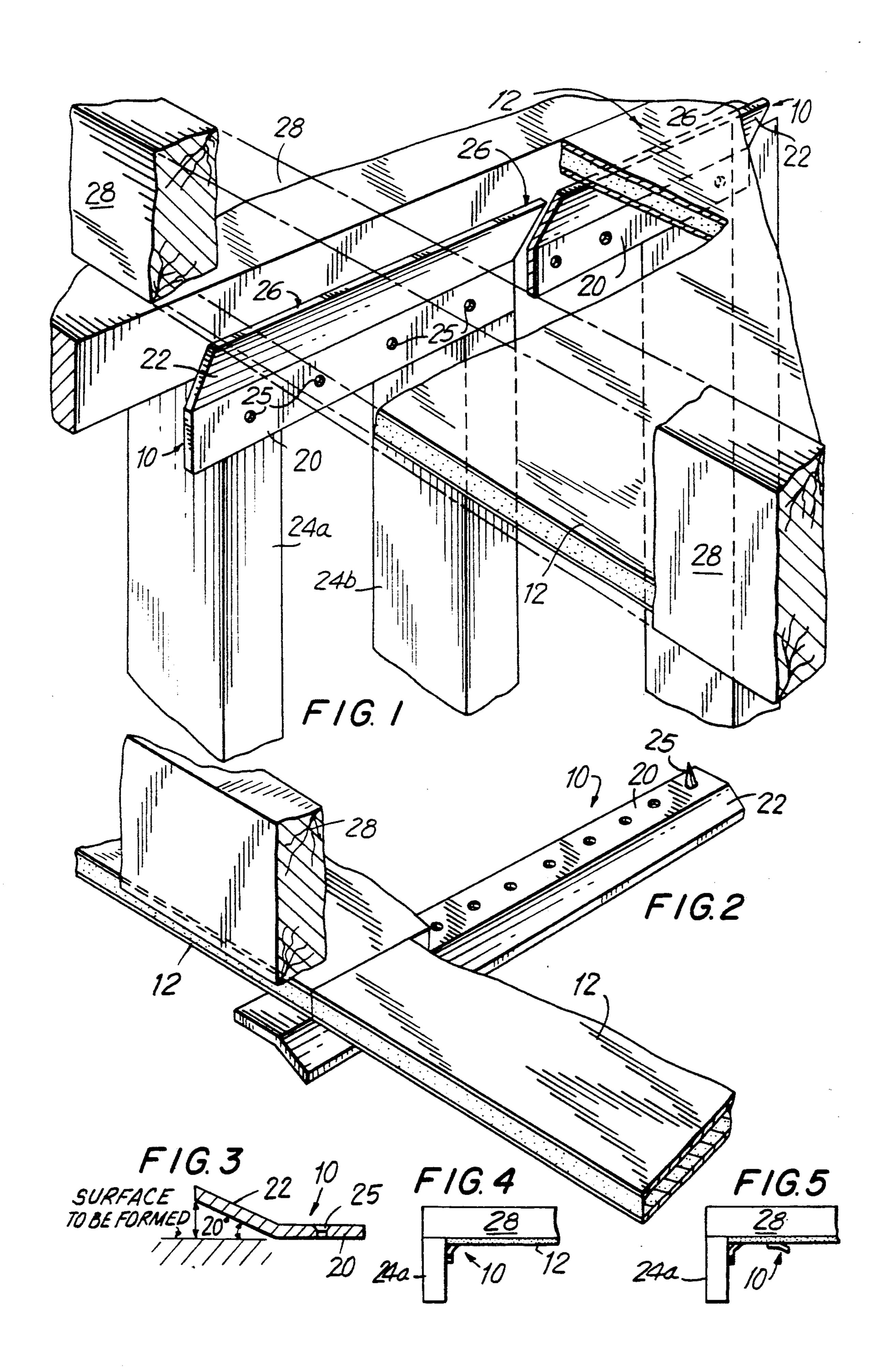
SLEEVE FOR AIDING IN THE AFFIXATION OF BOARD ON A SURFACE
