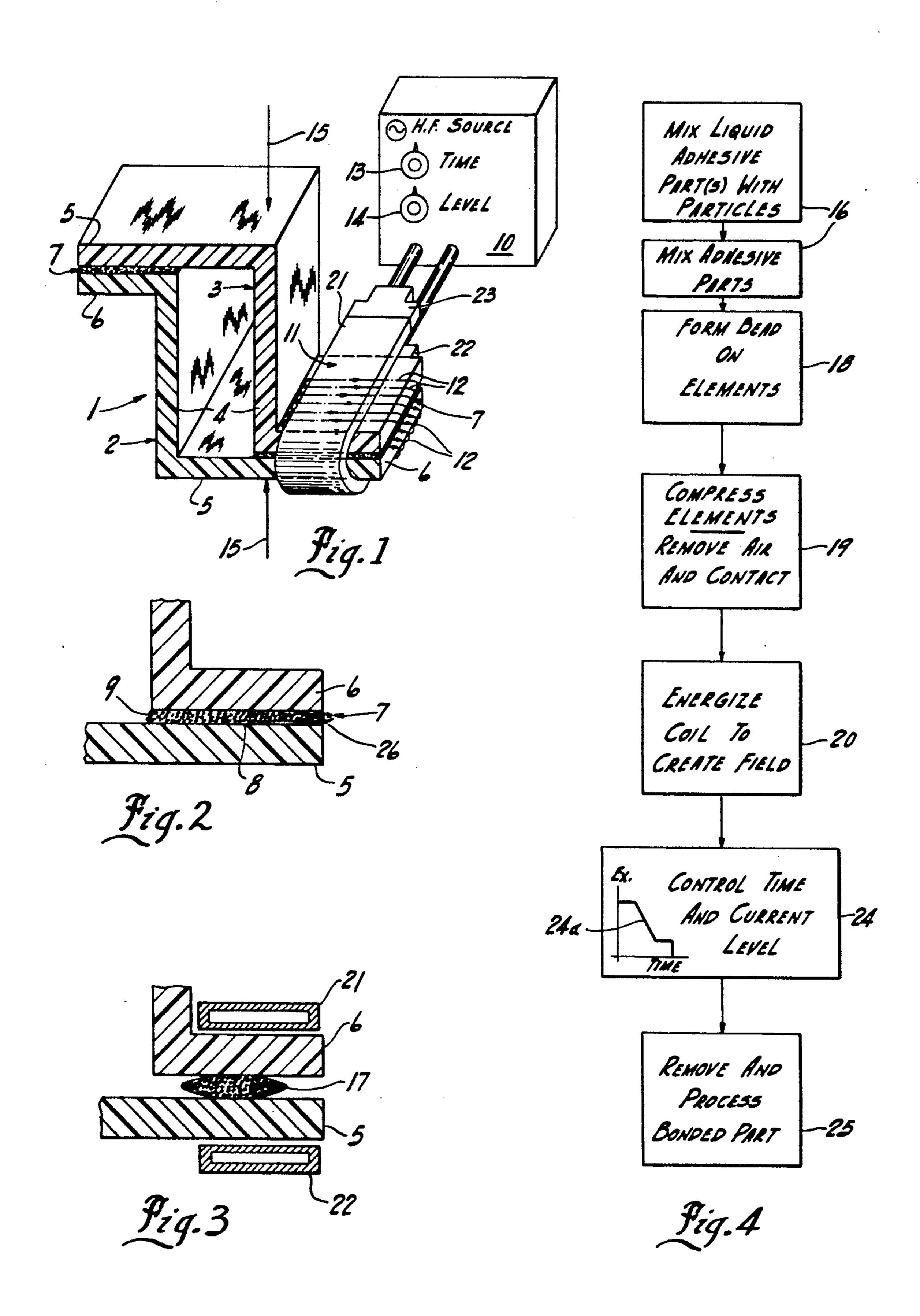
METHOD OF CURING THERMOSET BONDING AGENT FOR NON-DISTORTION SELF-SUPPORTING THERMOSET COMPONENT **PARTS**
