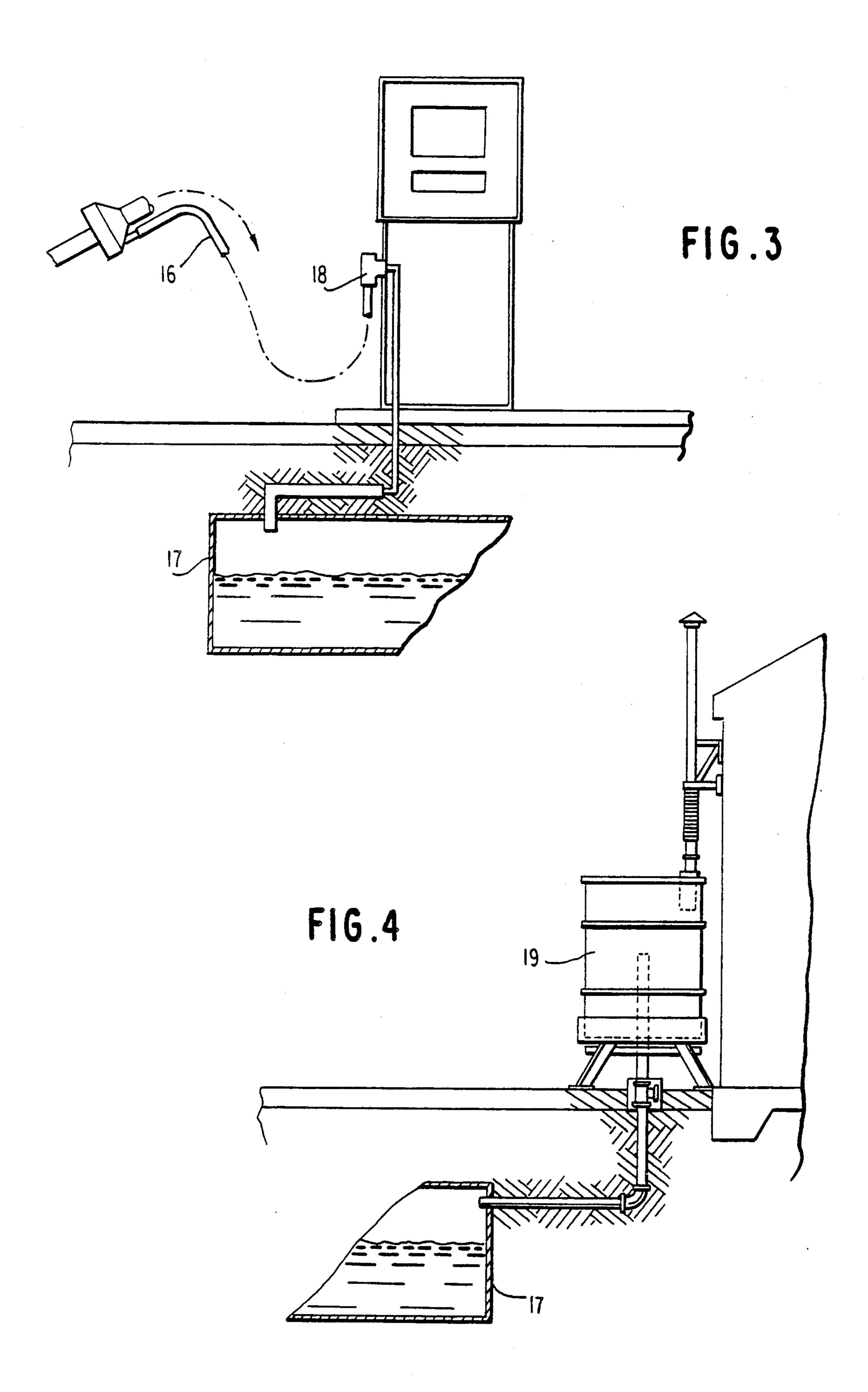
VAPOR COLLECTION ASSEMBLY FOR FUEL trolled. DISPENSING NOZZLE
