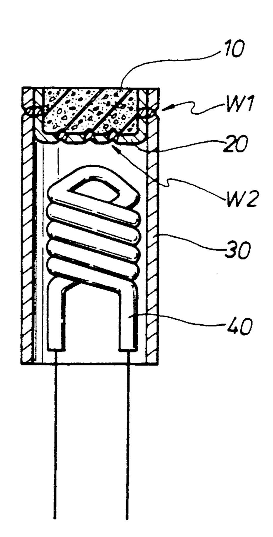
secure the parts. In particular, if the metal matrix is not completely secured, it is apt to come out of the cup.
