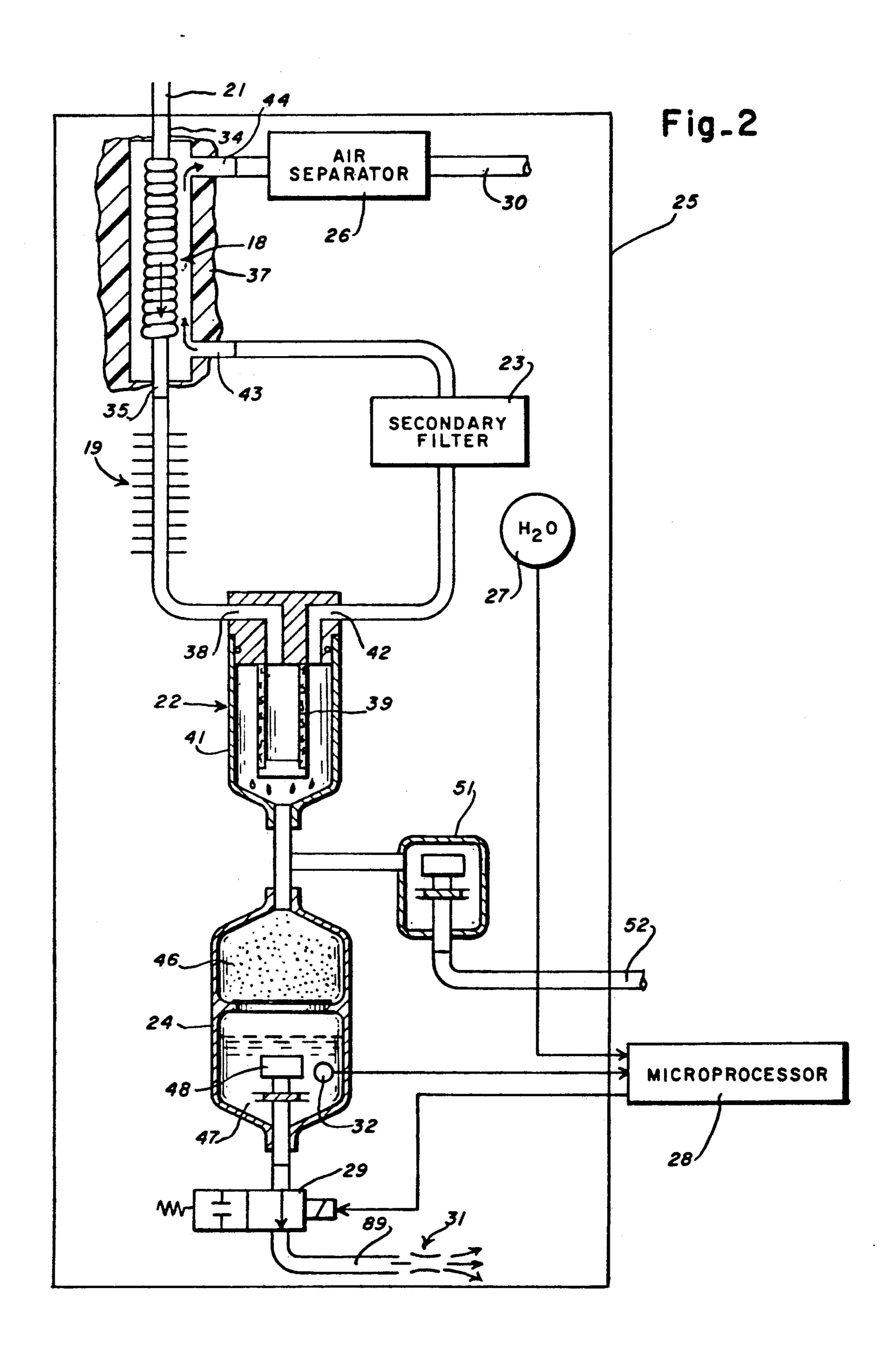
from a separation unit is humidified using condensate reclaimed from the compressed air line.
