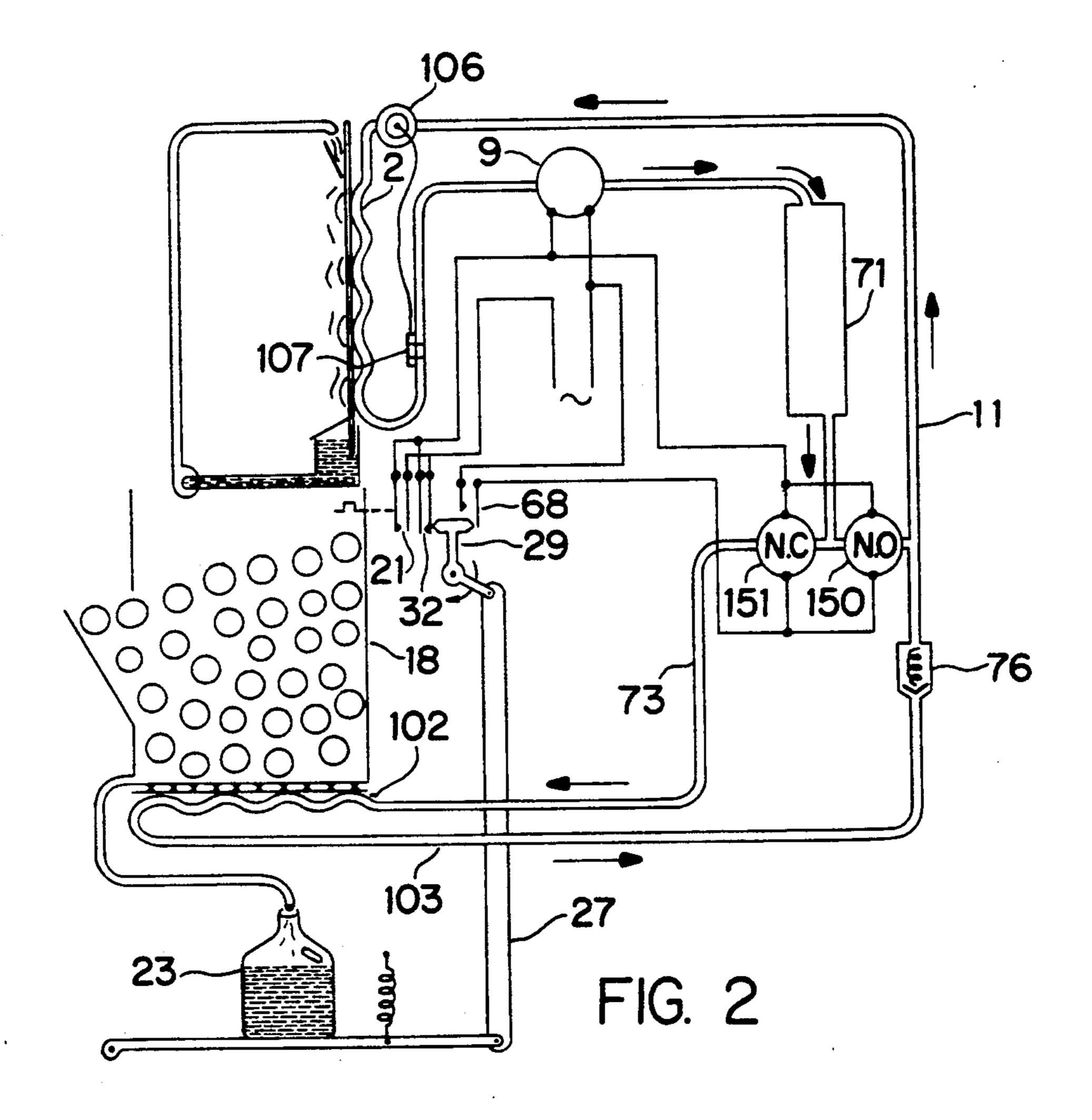
to shut off flow to the ice-melting condenser and to bypass liquid refrigerant flow back to the evaporator.
