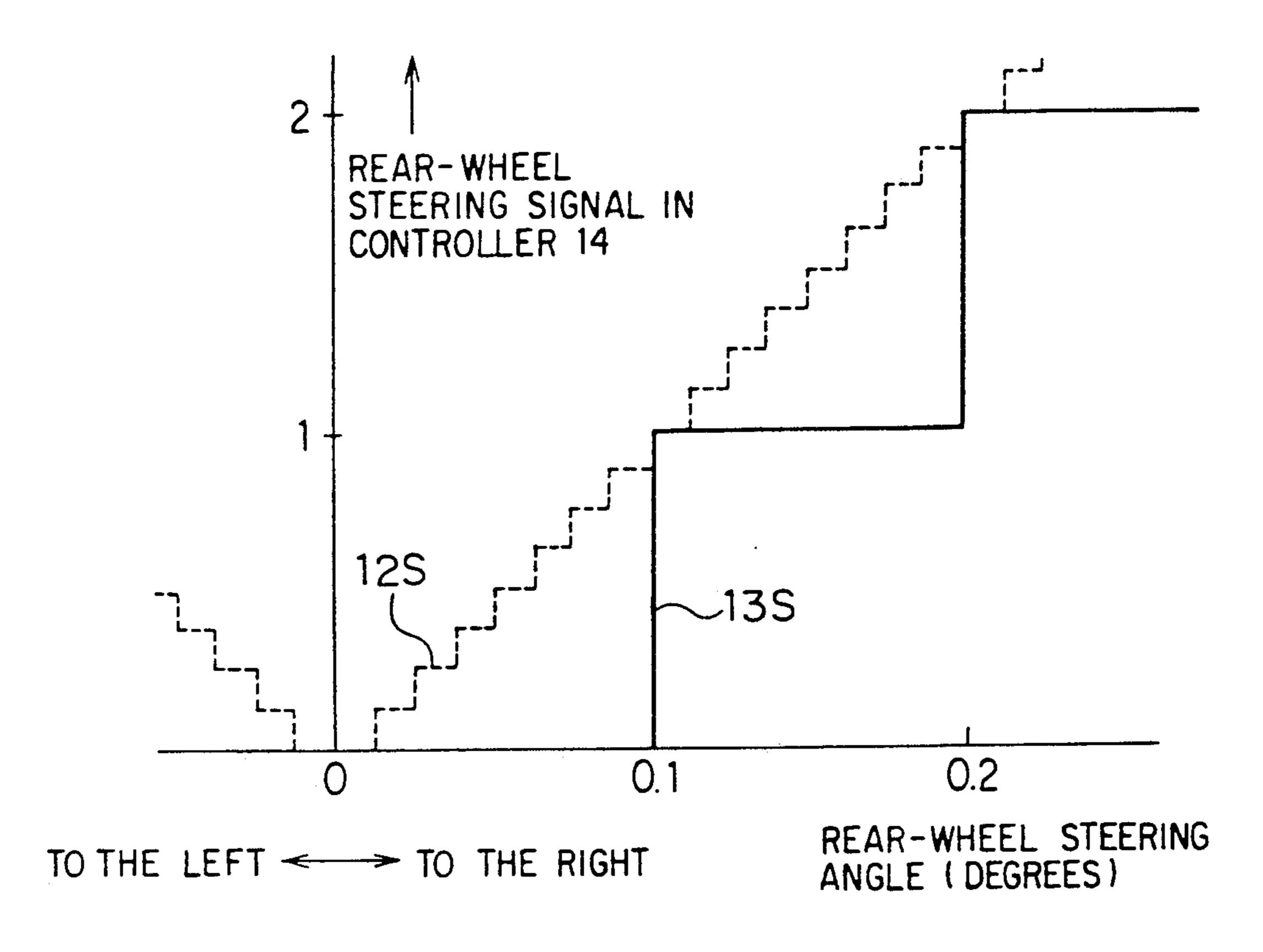
12S: OUTPUT SIGNAL OF PULSE GENERATOR 12
