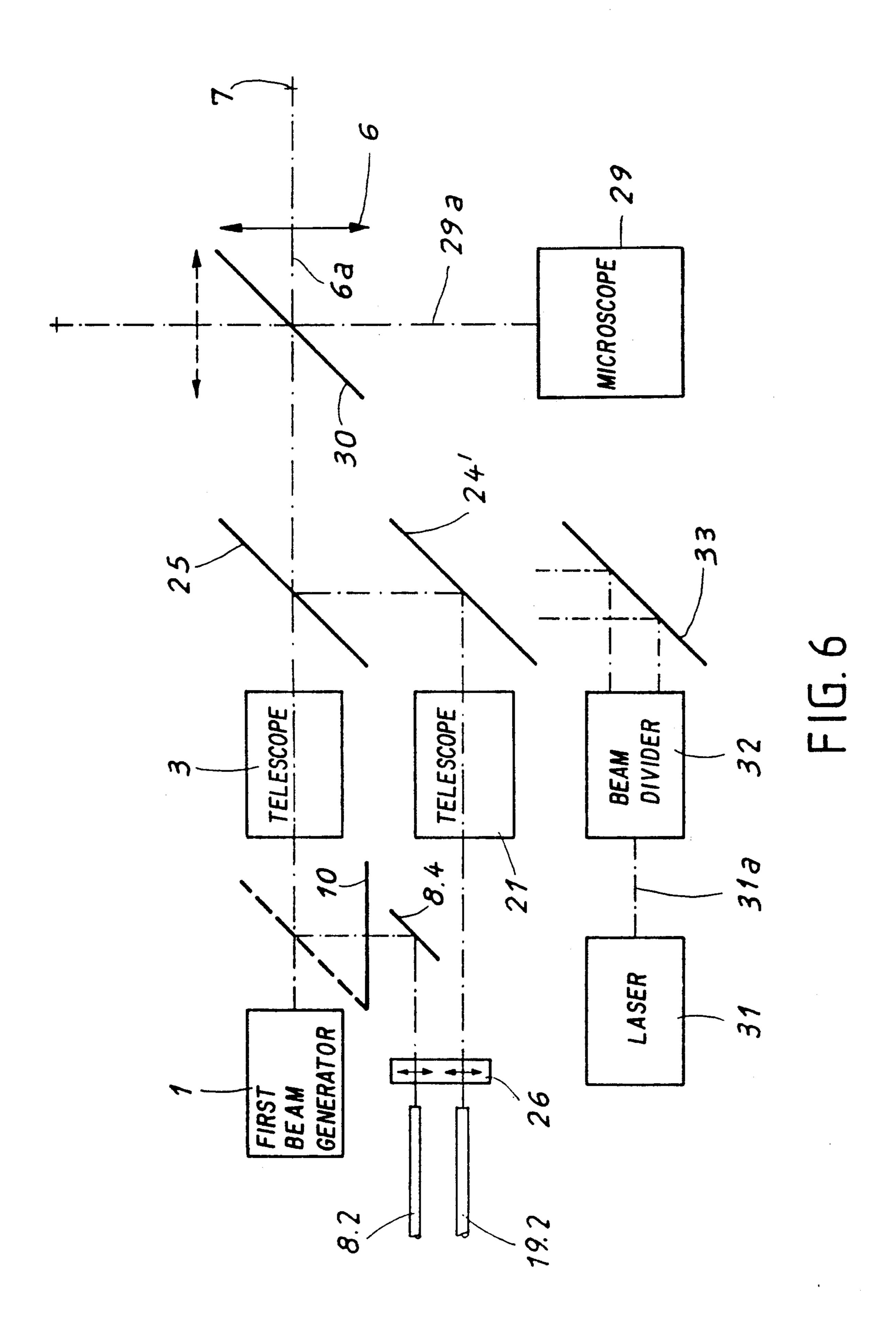
APPARATUS FOR THE SURGICAL TREATMENT OF A POINT SITUATED IN AN EYE
