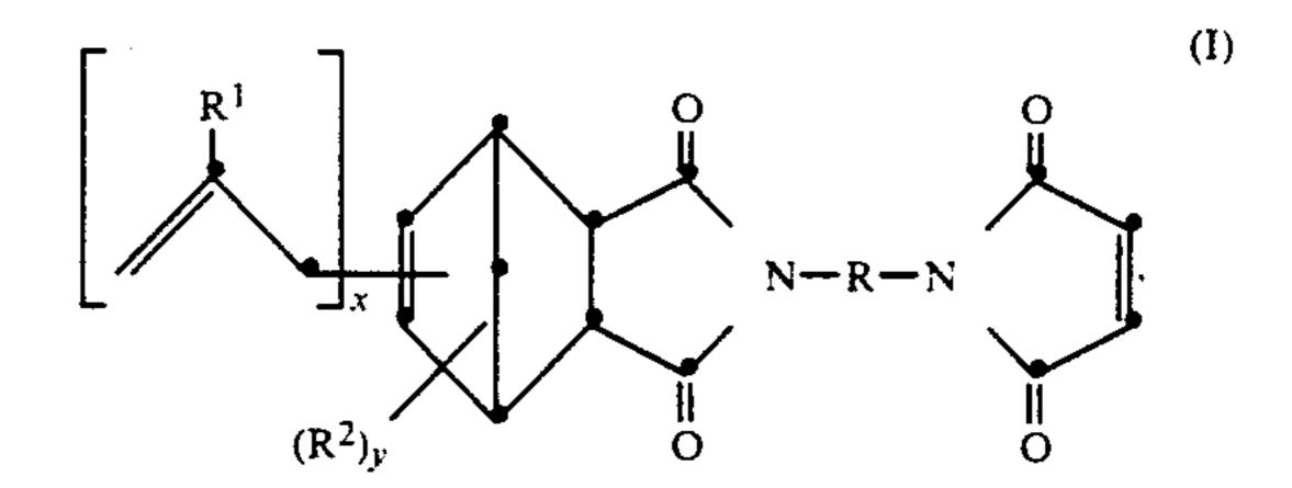
in which, for example, R<sup>1</sup> is hydrogen, x is 1, y is zero and R is bis-(1,4-phenylene)-methane are intermediates for the preparation of polymers having excellent physical properties, and are suitable for the production of mouldings, coatings and adhesive joints and, in particular, for the production of prepregs and heat-resistant composite materials.
