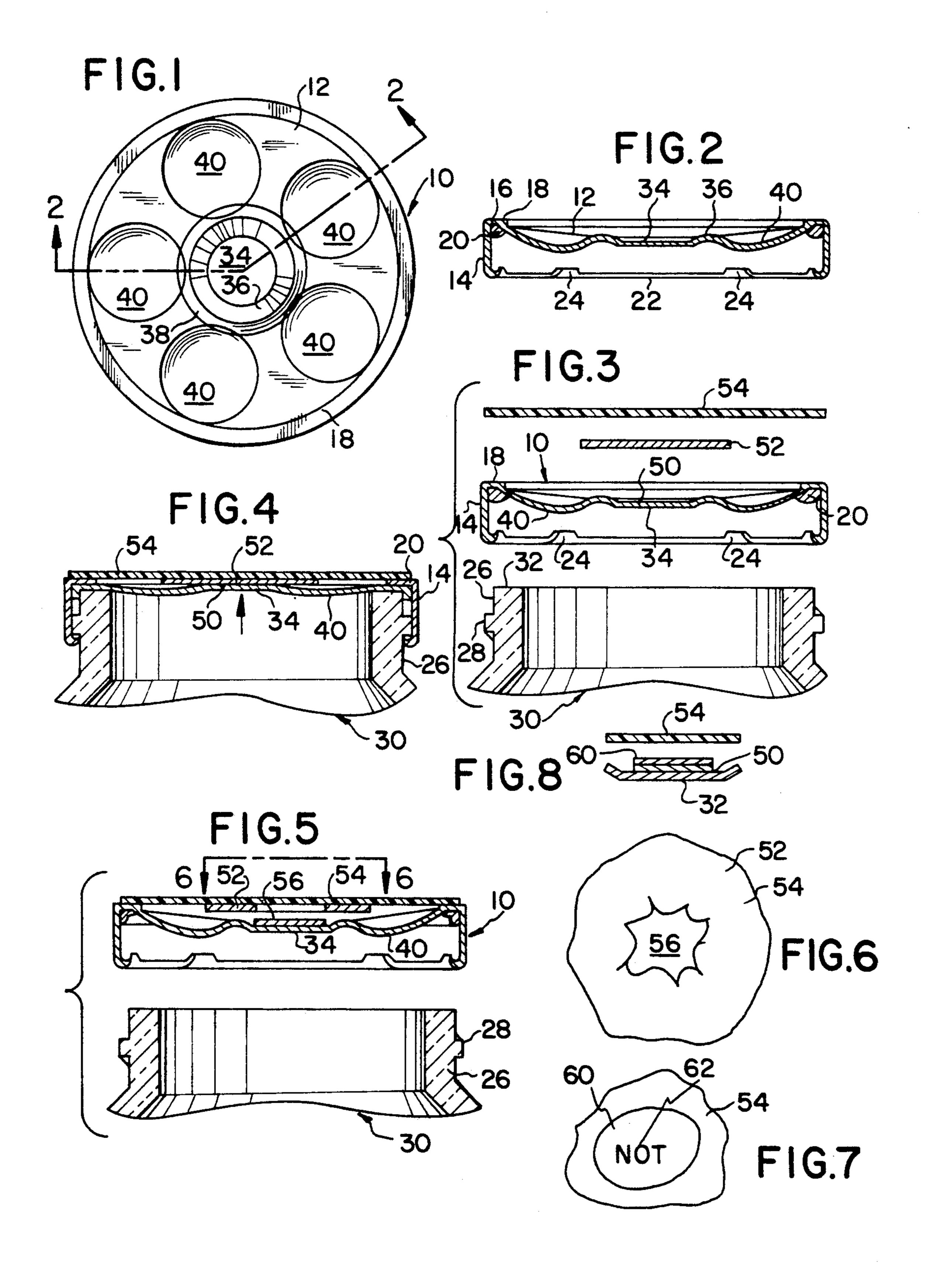
FIG. 4 is a vertical sectional view taken through the closure with the tamper indicating means applied
