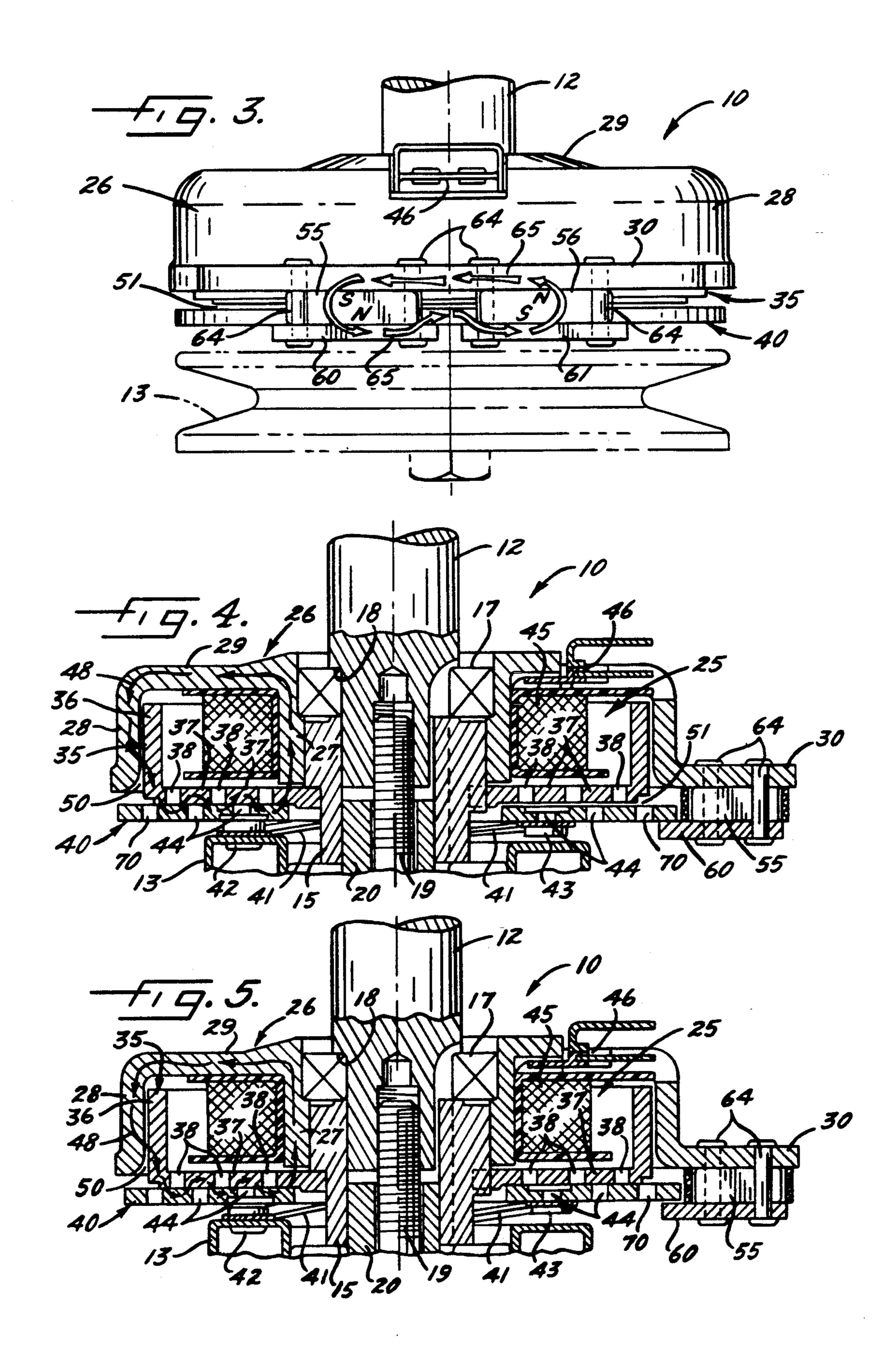
magnets which eliminate the need of strong springs for applying the brake.
