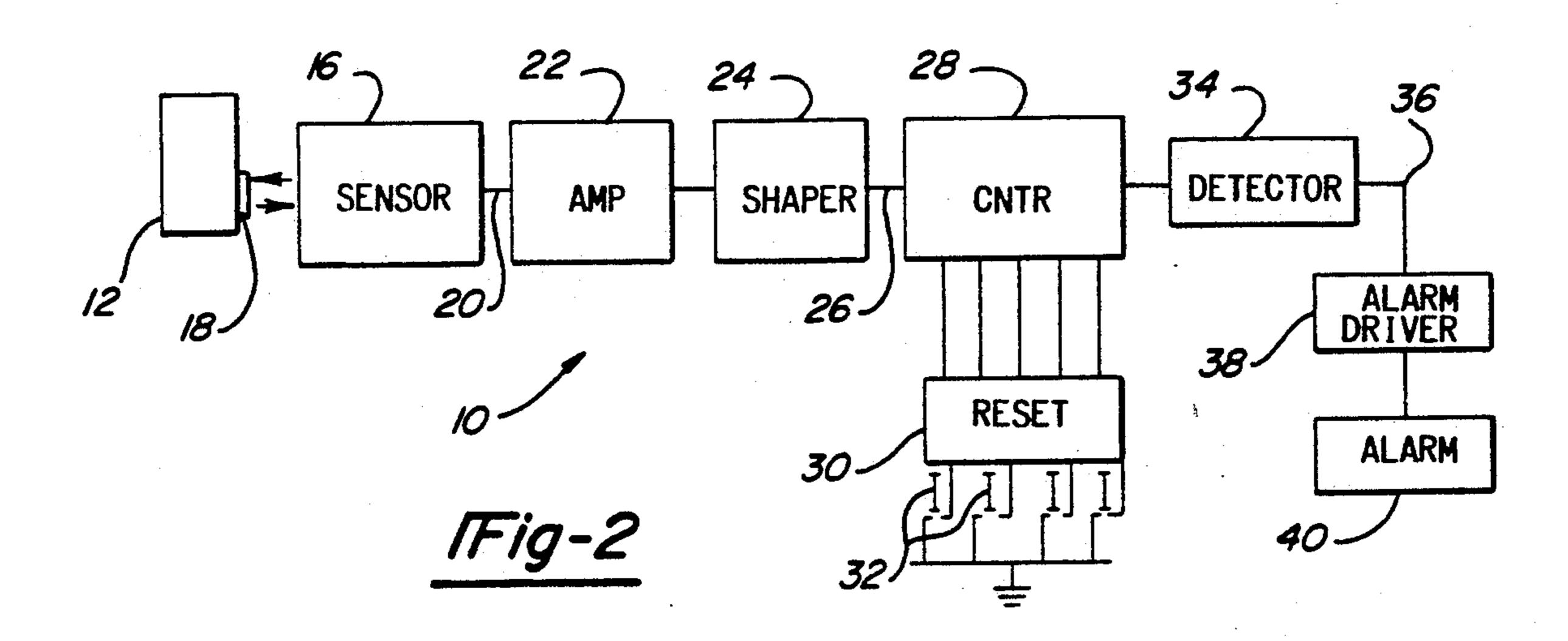
detector generates an output signal which activates an alarm.
