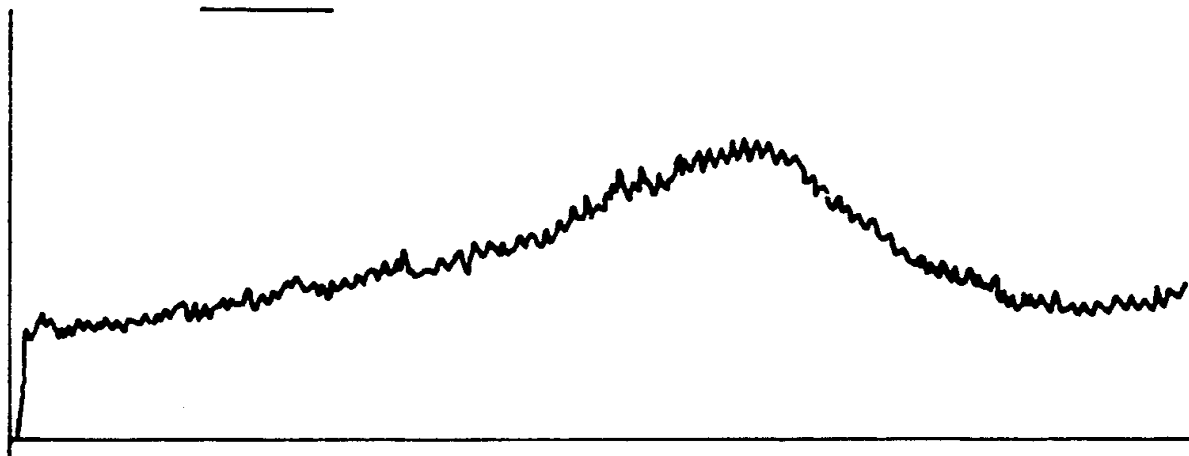
X-RAY DIFFRACTION SPECTRUM OF AMORPHOUS ERYTHROMYCIN ETHYLSUCCINATE AFTER 20 MONTHS OF CONSERVATION.
