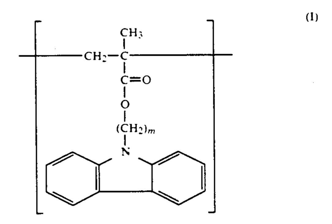
where m is an integer of from 3 to 11. The novel methacrylate (co)polymers containing carbazolyl side groups can advantageously be used as photoconductors in photoconductive layers, in particular of electrophotographic recording elements.
