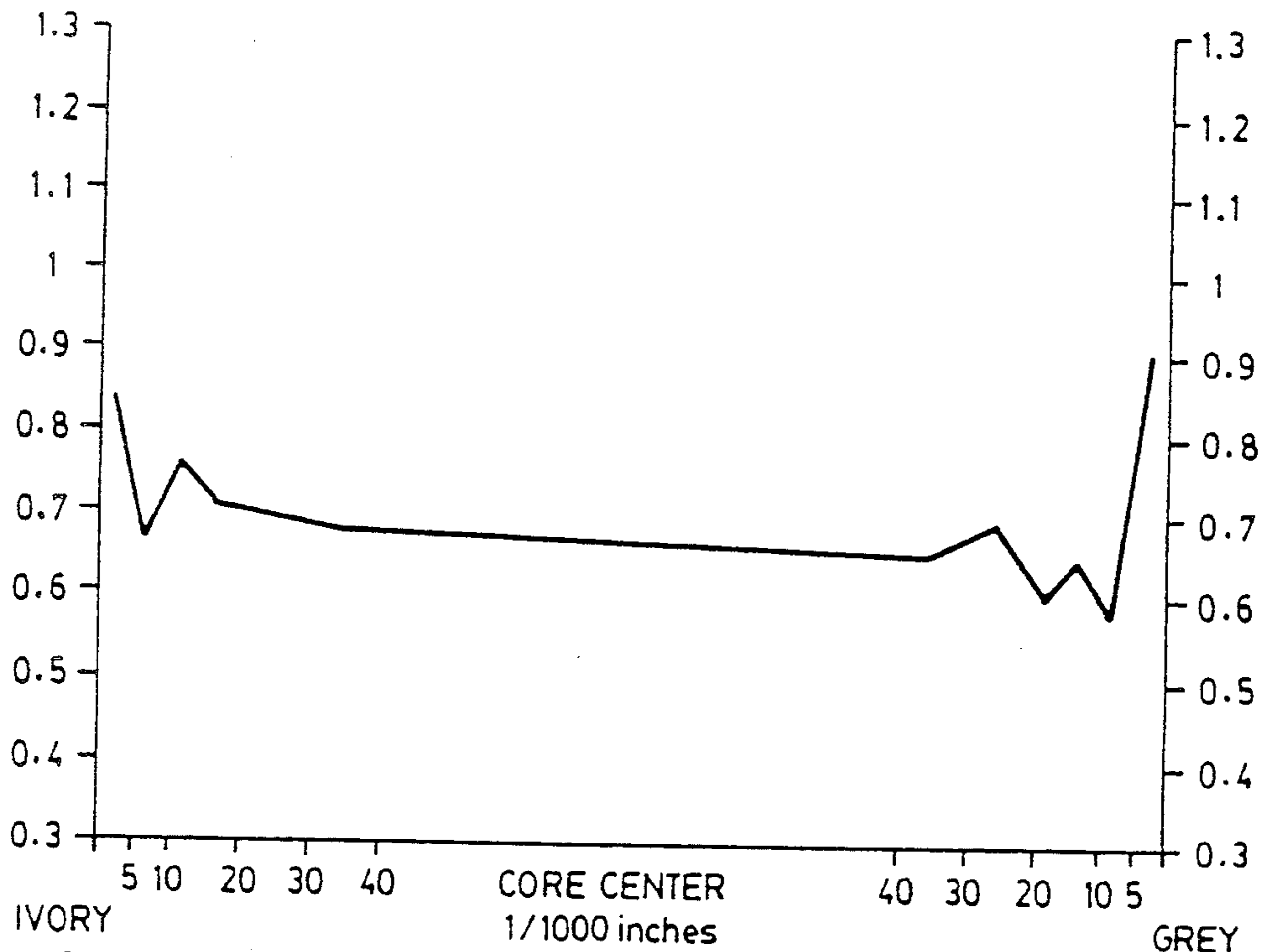
GYPSUM BOARD CORE SPECIFIC GRAVITY PROFILE
