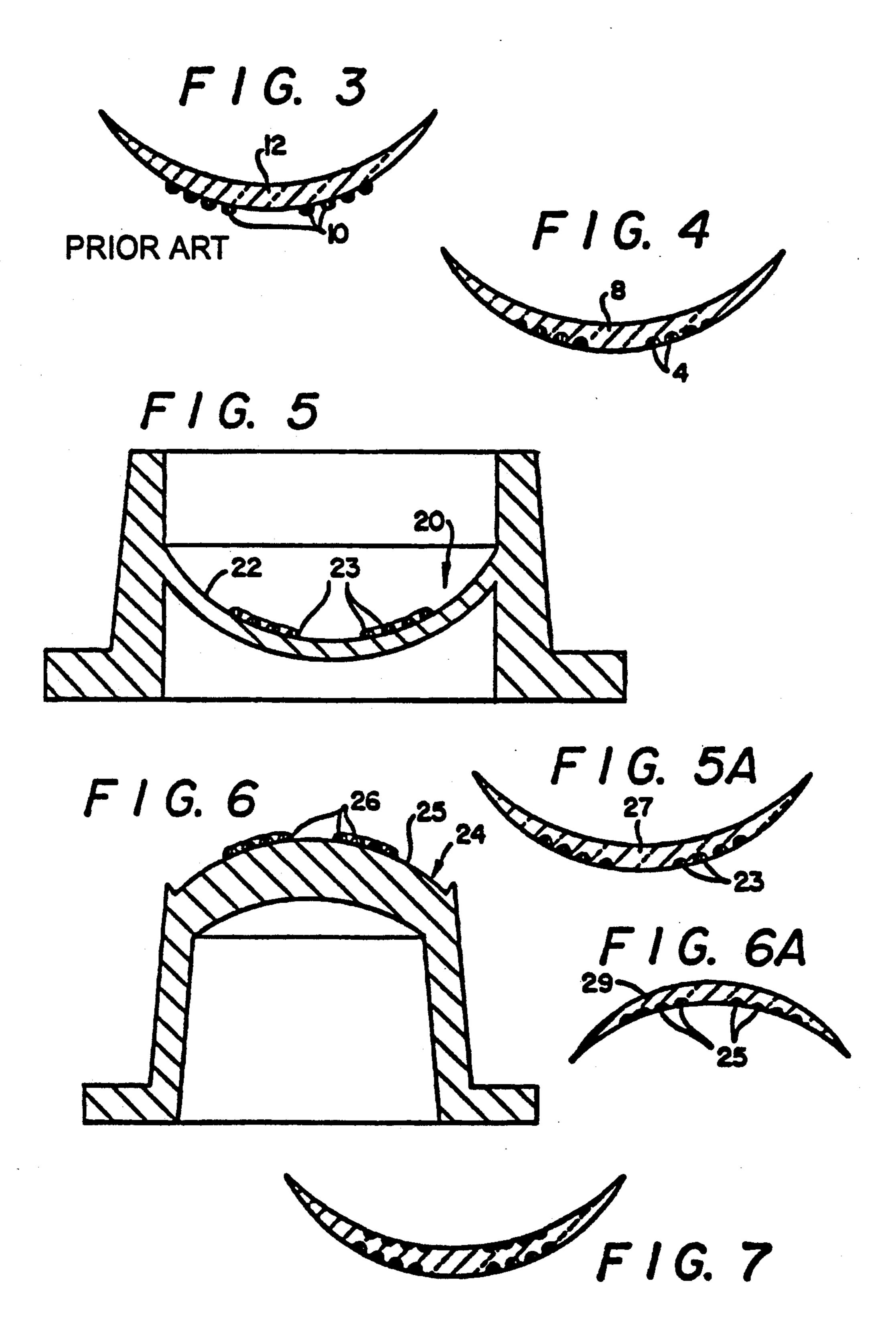
Consequently, the patentee employs rotational molding to cause a precipitated light absorbing material in the polymerizable mixture to be distributed to an annular zone about the vision region of the lens.
