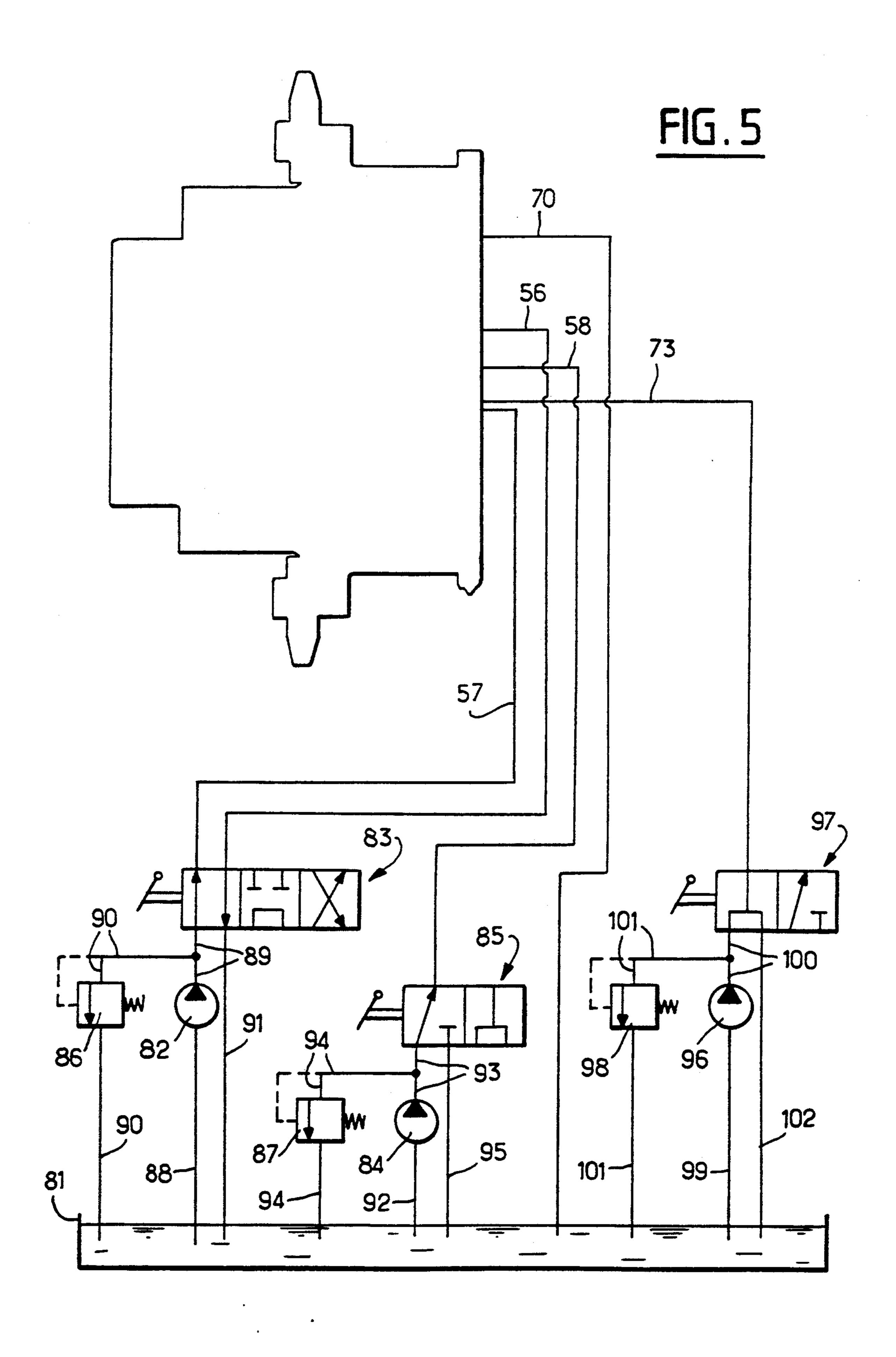
PRESSURE FLUID MECHANISM SUCH AS A MOTOR OR A PUMP COUPLED TO A BRAKING DEVICE
