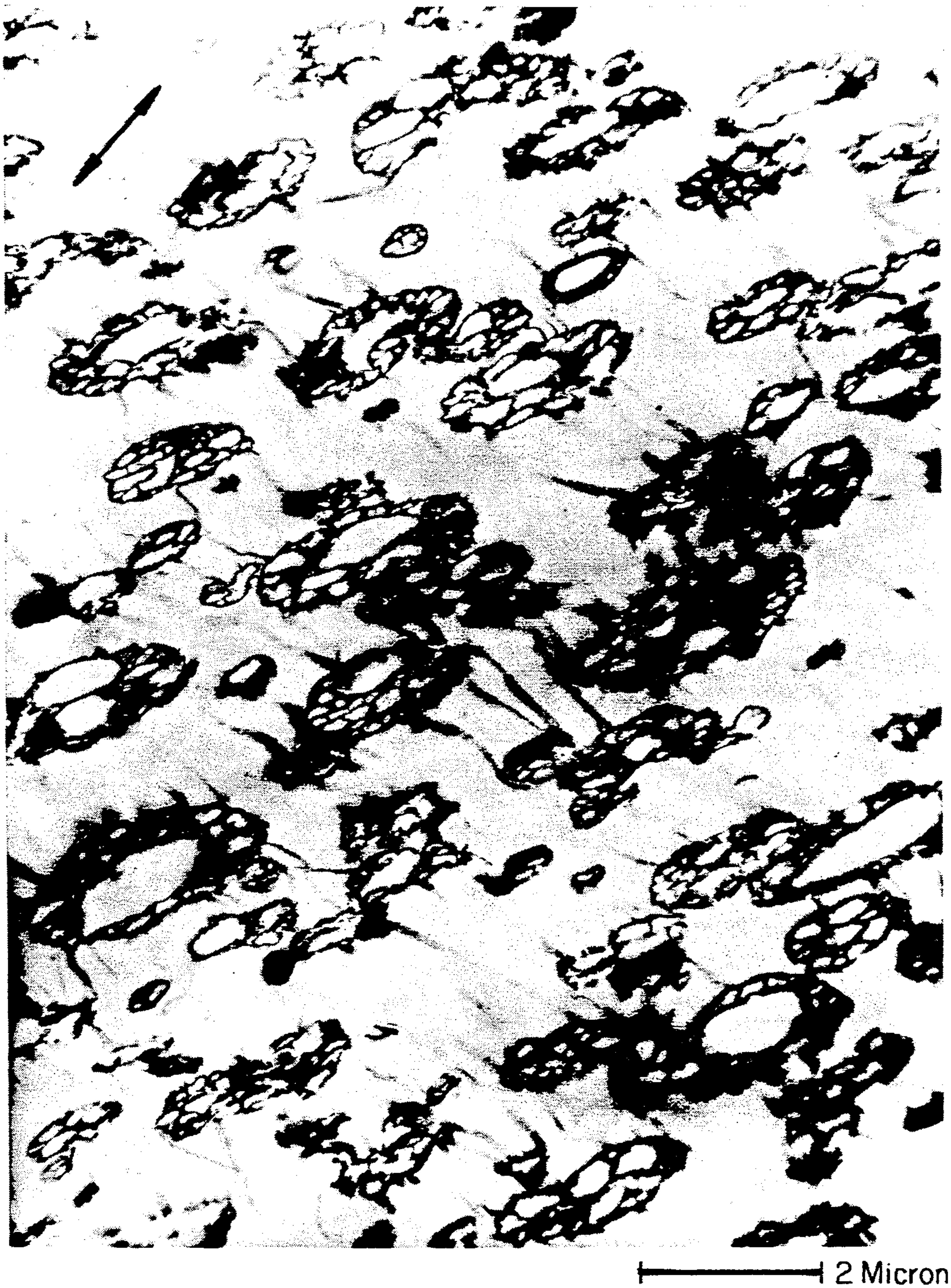
FIG. 18: TEM micrograph of the acrylonitrile-butadiene-styrene compression moulded film
