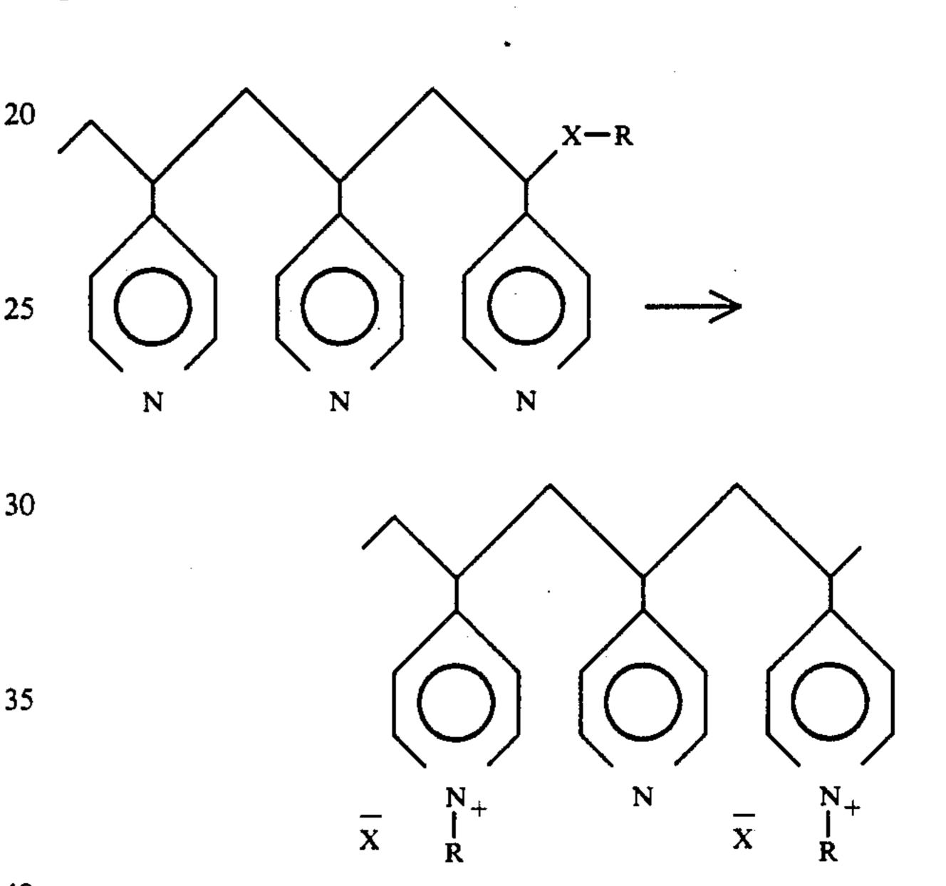
The poly(vinylpyridine) contained in a porous material is simultaneously charged and rendered insoluble by the cross linking reaction with a difunctional alkylating agent as schematically shown below.
