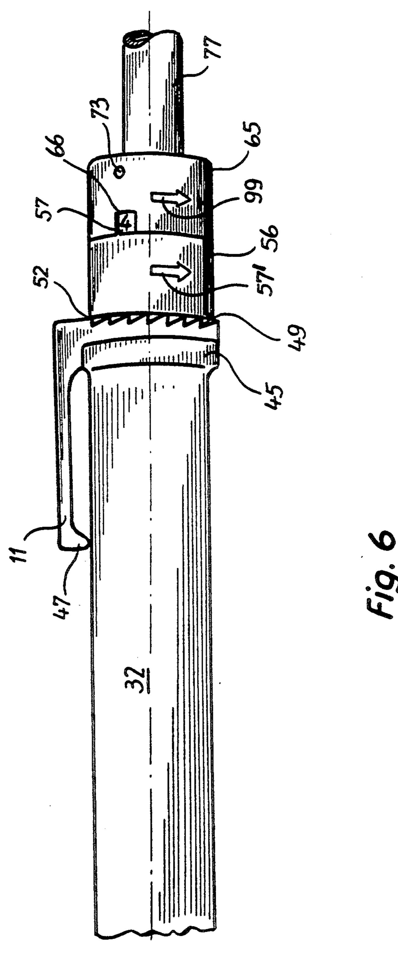
INJECTION DEVICE FOR INJECTION, ESPECIALLY SELF-ADMINISTERED INJECTION, OF MEDICAMENT, INCLUDING MECHANISMS FOR NULLING AND FOR SELECTING DOSAGE, ESPECIALLY FOR USE WITH MULTI-DOSE AMPULES
